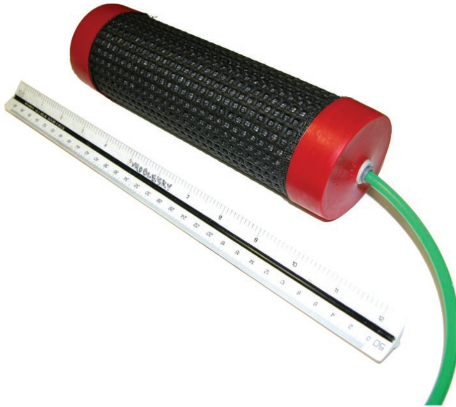
Figure 4. A 2.5-inch-diameter pore-water sampler with scale.
