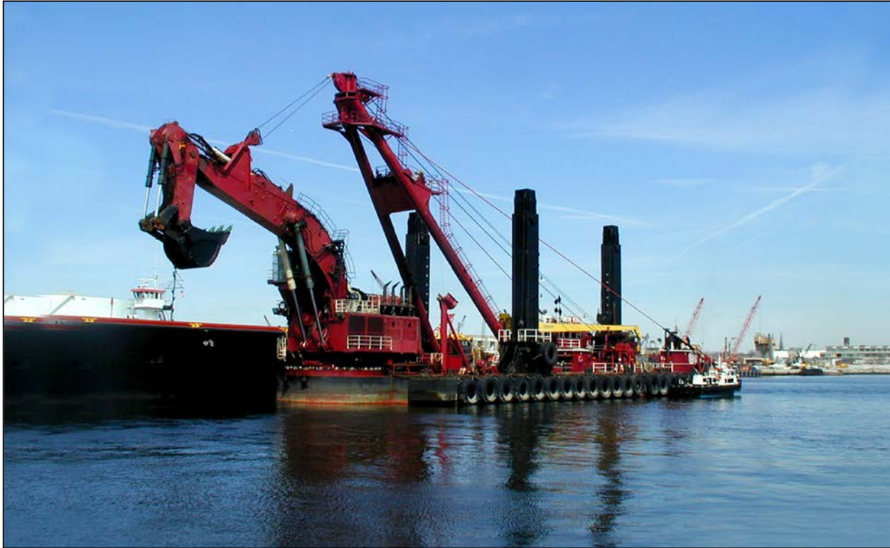
Figure 2-36 Backhoe Dredge New York (Courtesy of Great Lakes Dredge and Dock Company, Oak Brook, IL)
