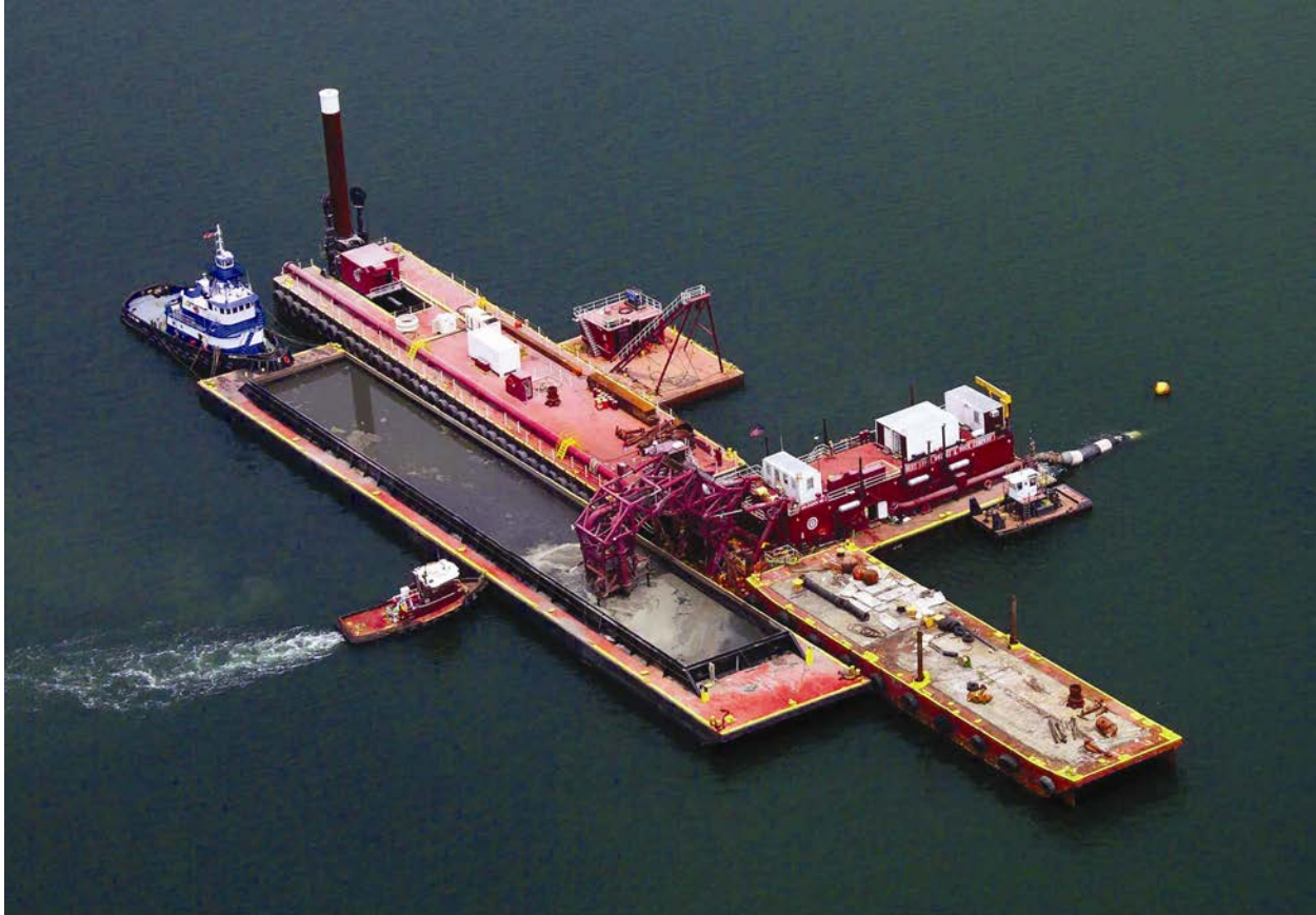
Figure 2-34. Hydraulic Unloader (Courtesy of Great Lakes Dredge and Dock Company, Oak Brook, IL)
