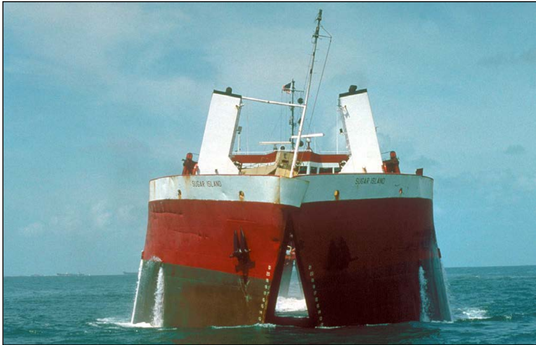
Figure 2-29. Split-Hull Hopper Dredge Unloading Dredged Material (Dredge Sugar Island , Great Lakes Dredge and Dock Company)
