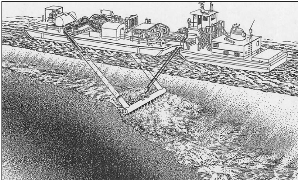
Figure 2-38. Water Injection Dredge
