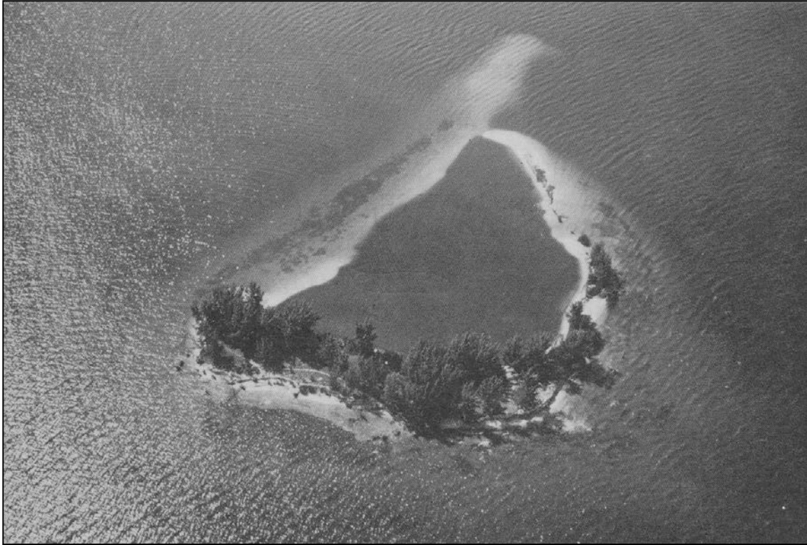
Figure 5-29. A Dredged Material Island in Florida, Typical of Those Built in the U.S. Intracoastal Waterway
