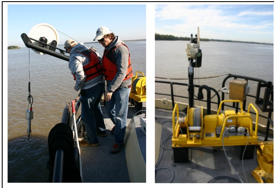
Figure 2-7. STEMA RheoTune Probe Being Deployed off the New Orleans District's S/V Teche via a Semi-Automated Winch
