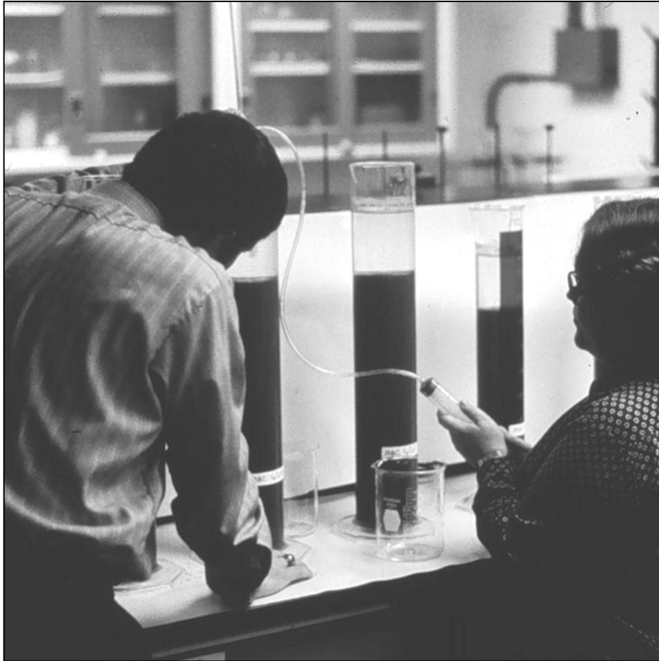
Figure 4-66. Modified Elutriate Test in Progress
