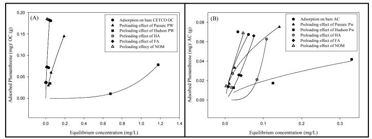
**Figure 7.1-17**. Effects of Passaic River sediment pore water, Hudson River sediment pore water, humic acid, fulvic acid and natural organic matter on the adsorption kinetics of phenanthrene by (A) organoclay and (B) activated carbon.
