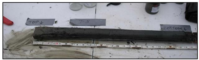
**Figure I-6**. Sediment core collected at control area T5 (no treatment).
