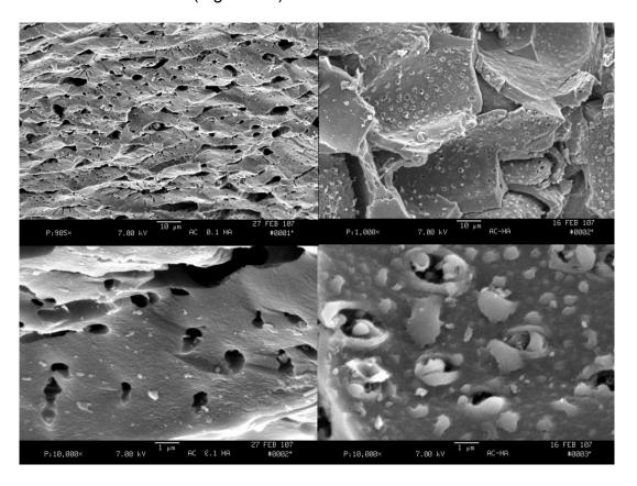
Figure 2.2: Comparative SEM image for coconut shell AC preloaded with 0.1 g/L humic acid solution (upper and bottom left) and coconut shell AC preloaded with 1 g/L (upper and bottom right).
