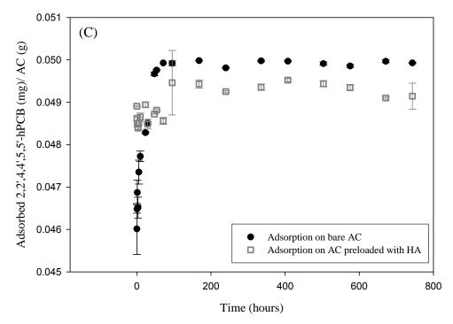
Figure 2.3: Kinetics of adsorption of PCB congeners on coconut shell AC in presence and absence of HA: (B) 2, 2', 5, 5'-tetrachlorobiphenyl and (C) 2, 2', 4, 4', 5, 5'-hexachlorobiphenyl.
