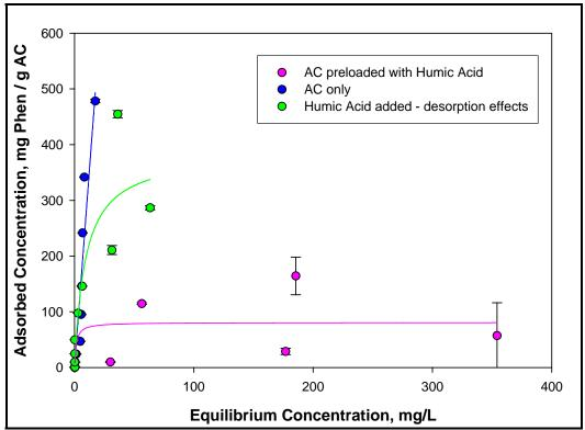
**Figure 7.1-15.** Adsorption isotherm for phenanthrene onto activated carbon.
