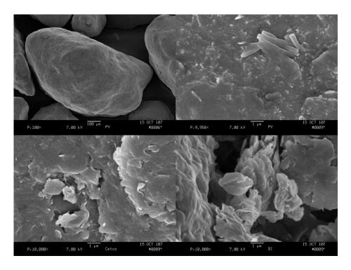
Figure 3.1.1: Surface profiles of organoclays: Polymer Ventures (100 x magnification – top left and 10 K x magnification - top right); CETCO (10K x magnification - bottom left) and Biomin Inc. (10K x magnification - bottom right)
