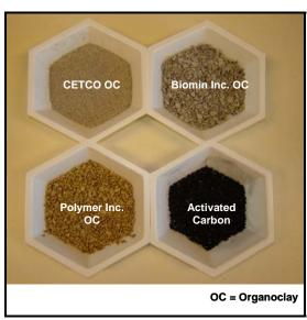
**Figure 6.1-1.** Reactive capping materials for organic contaminant sequestration.
