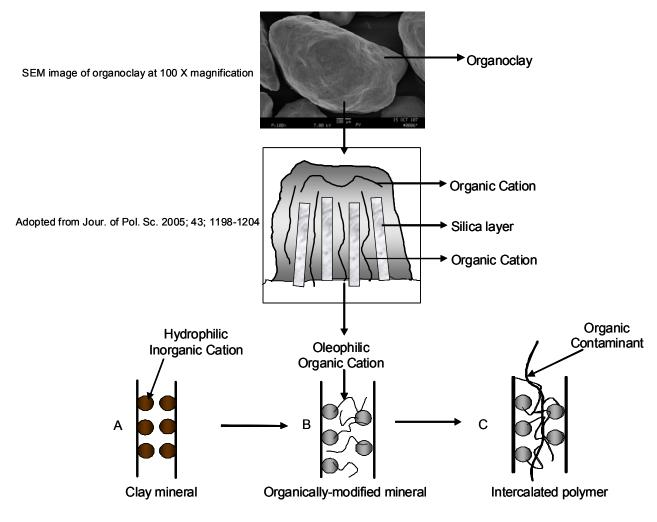
Mechanism of sorption onto organoclay
