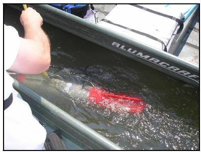
Figure 6.2-2. Side-scan sonar transducer ("fish") deployed from dual jon-boat survey craft.
