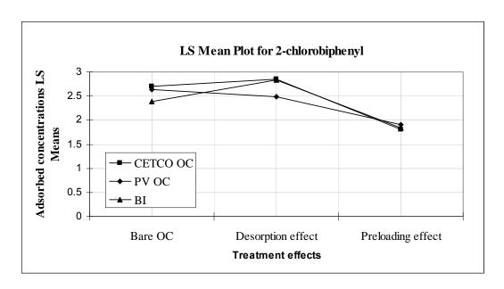
Figure 3.4: Least square means plot for adsorption of 2-chlorobiphenyl on all the three organoclays
