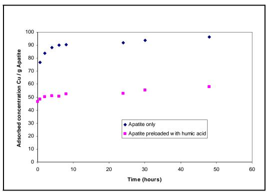
Figure 7.1-6. Kinetics of copper adsorption on apatite.
