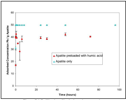
Figure 7.1-7. Kinetics of lead adsorption on apatite.
