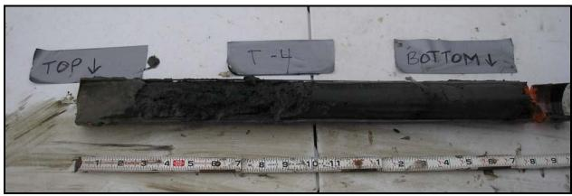
Figure I-5. Sediment core collected at treatment area T4 (sand cap only).
