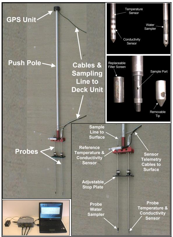
**Figure 6.2-5**. Complete Trident probe system showing the conductivity and temperature sensor, water sampling probe, push-pole, GPS unit and deck unit.
