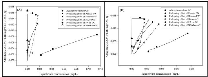
**Figure 7.1-15**. Effects of Passaic River sediment pore water, Hudson River sediment pore water, humic acid, fulvic acid and natural organic matter on the adsorption kinetics of 2,2',5,5'-tetrachlorobiphenyl by (A) organoclay and (B) activated carbon.
