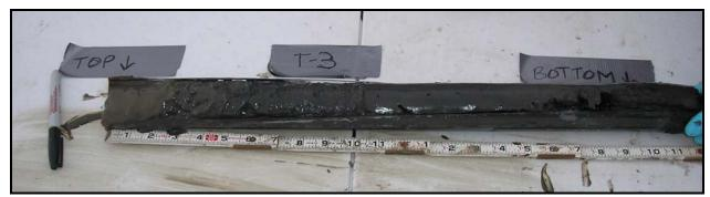
**Figure I-4**. Sediment core collected at treatment area T3 (double mat).
