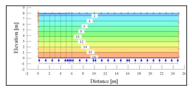
**Figure C-7**. Pressure head contours (m) and flow paths ( $k_{GT} = 0.1 \text{ x } k_{SED}$ ).
