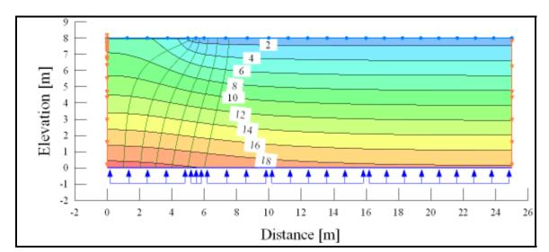
**Figure C-10**. Pressure head contours (m) and flow paths ( $k_{GT} = 0.0001 \text{ x } k_{SED}$ )
