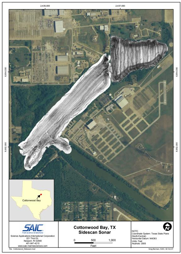
Figure 7.2-8. Complete side-scan sonar results for Cottonwood Bay.
