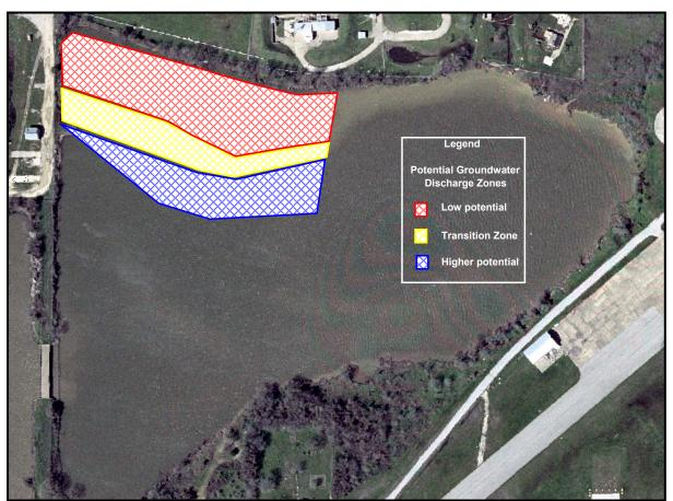
Figure 7.2-16. Potential groundwater discharge zones for Cottonwood Bay.
