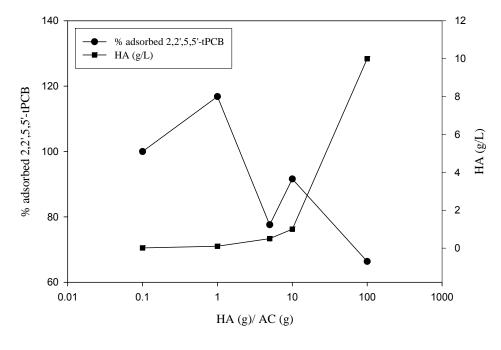
Figure 2.9: Effect of different loadings of HA on coal based activated carbon
