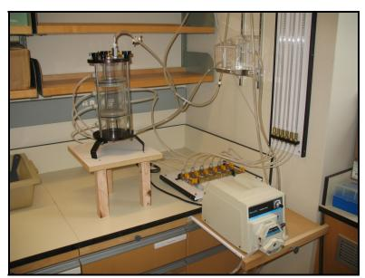
**Figure 6.3-4.** Geotextile permeability column experimental setup.
