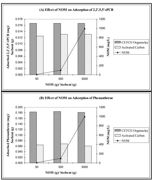
**Figure 7.1-22**. Effects of different loading levels of natural organic matter on the adsorption kinetics of organoclay and activated carbon for (A) 2,2',5,5'-tetrachlorobiphenyl and (B) phenanthrene.
