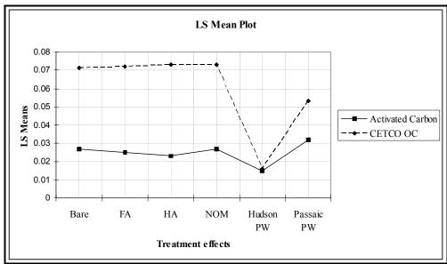
**Figure 7.1-18**. Least square mean plot to compare the effects of Passaic River sediment pore water, Hudson River sediment pore water, humic acid, fulvic acid and natural organic matter on the adsorption of phenanthrene by organoclay and activated carbon.
