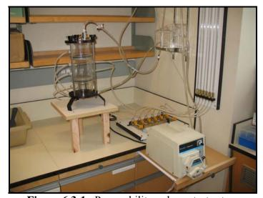
**Figure 6.3-1.** Permeability column test setup.
