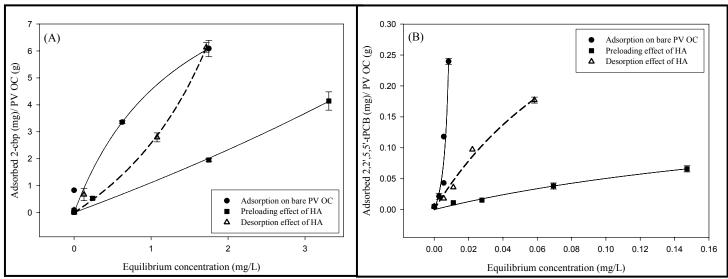
**Figure 7.1-10**. Langmuir isotherms for adsorption of two selected PCB congeners on bare Polymer Ventures organoclay with preloading and desorption effects of humic acid: (A) 2-chlorobiphenyl and (B) 2,2',5,5'-tPCB.
