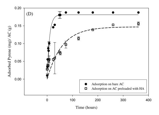
Figure 4.1 D: Kinetics: Pyrene adsorption on activated carbon
