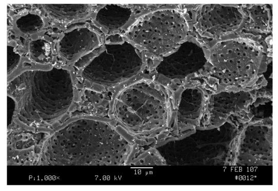
Coconut shell activated carbon: 1000 x magnifications
