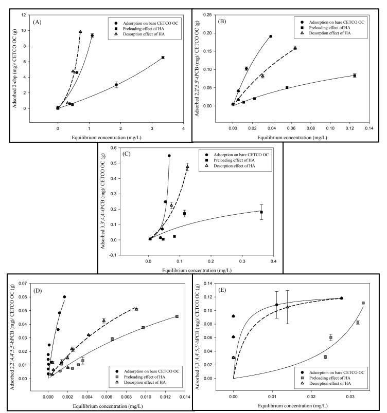
**Figure 7.1-9**. Langmuir adsorption isotherms for five PCBs on bare CETCO organoclay with preloading and desorption effects of humic acid: (A) 2-cbp, (B) 2,2',5,5'-tPCB, (C) 3,3',4,4'-tPCB, (D) 2,2',4,4',5,5'-hPCB and (E) 3,3',4,4',5,5'-hPCB.
