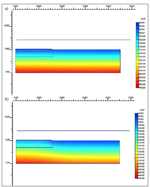
**Figure 7.3-10**. Total water pore pressure for an unclogged mat (a) and a clogged mat (b) under the uncoupled seepage model.
