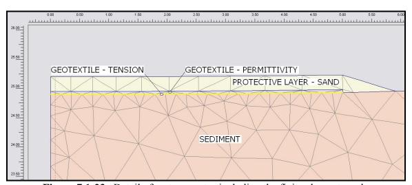
Figure 7.1-23. Detail of mat geometry including the finite element mesh.
