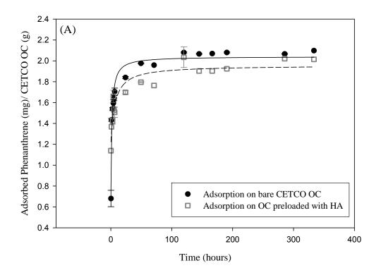
Figure 4.1A: Kinetics: Phenanthrene adsorption on organoclay
