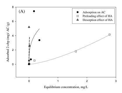
Figure 2.4 A. Freundlich Adsorption Isotherms for selected PCB congeners with bare AC and preloading and desorption effect of HA: 2-chlorobiphenyl
