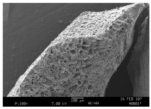
Coconut shell activated carbon: 100 x magnifications
