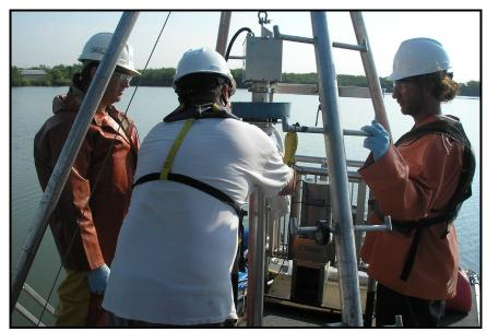
Figure 6.2-4. Vibe-Core-D coring apparatus deployed through moon pool of pontoon boat.
