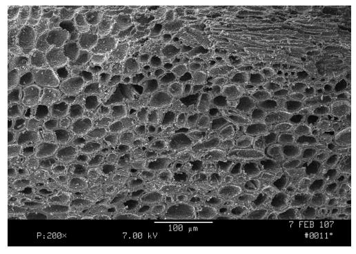
Coconut shell activated carbon: 200 x magnifications
