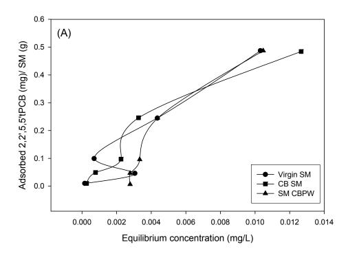
Figure 5.5 A: Comparison of bare sorbent mixture with the sorbent mixture obtained from reactive core mats deployed in Cottonwood Bay for 6 months: 2, 2', 5, 5'-tPCB adsorption(SM = Sorbent mixture; CB = Cottonwood Bay; and PW = Porewater)
