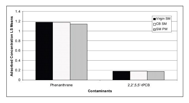
Figure 5.6: Statistical analysis of performance of sorbents: 2, 2', 5, 5'-tPCB and phenanthrene adsorption on SM and CB SM (SM = Sorbent Mixture, CB = Cottonwood Bay and PW = Porewater)
