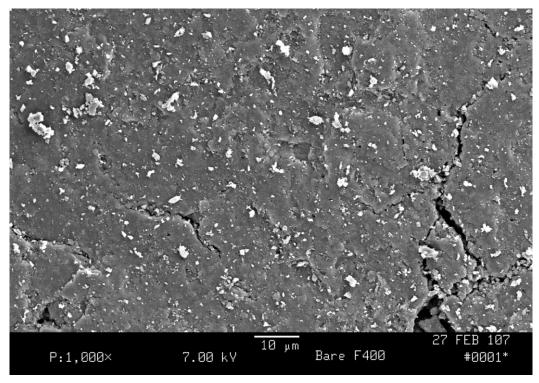
Coal based activated carbon: 1000 x magnifications
