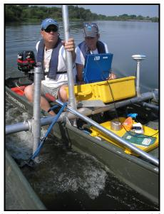
Figure 6.2-1. Bathymetry and sub-bottom transducer deployed from dual jon-boat survey craft.
