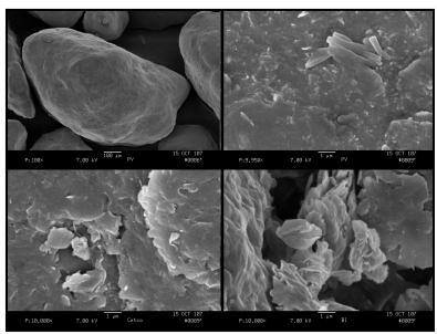
**Figure 6.1-1.** Scanning electron micrograph surface profiles of three different organoclays: Polymer Ventures (100x magnification - top left and 10K x magnification - top right), CETCO (10K x magnification - bottom left) and Biomin, Inc. (10K x magnification - bottom right).
