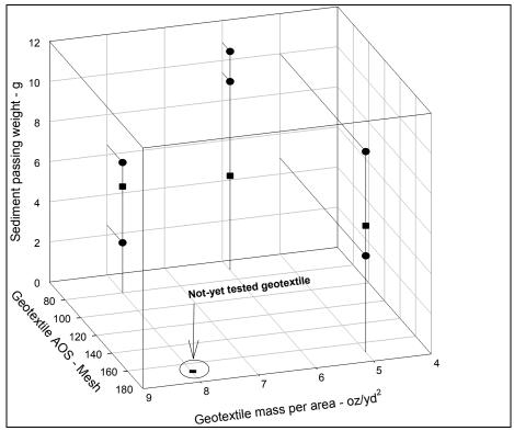
Figure 7.3-5. Weight of sediment passing through each geotextile during the gradient ratio tests.
