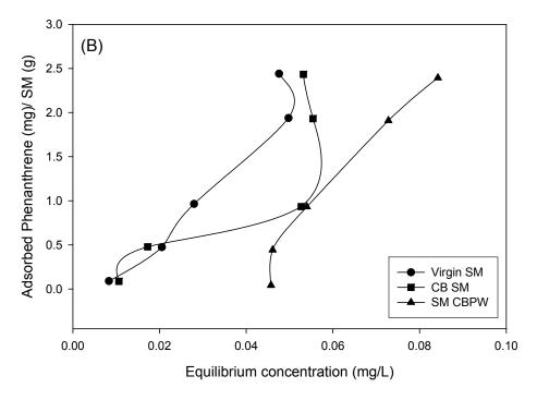
Figure 5.6B: Comparison of bare sorbent mixture with the sorbent mixture obtained from reactive core mats deployed in Cottonwood Bay for 6 months: Phenanthrene adsorption (SM = Sorbent mixture; CB = Cottonwood Bay; and PW = porewater)
