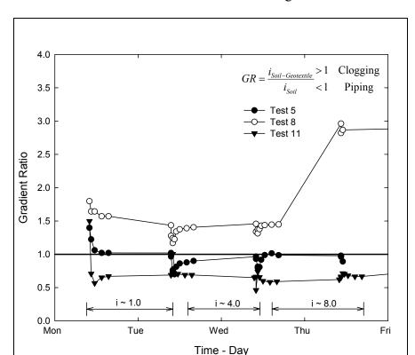
The gradient ratio value over time obtained for the CETCO 3 geotextile is shown in Figure 7.3-3.
