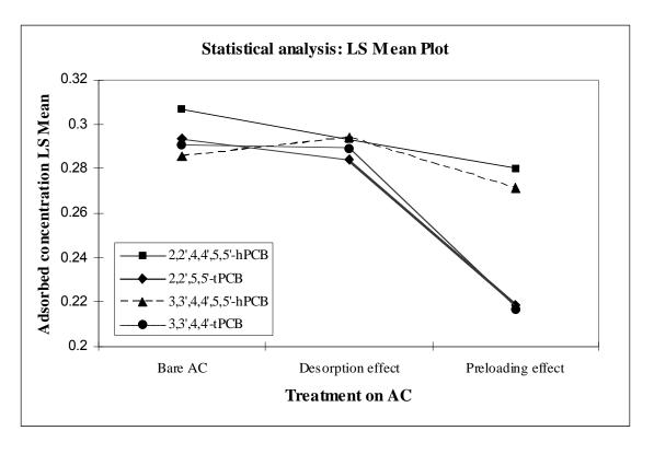
Figure 2.5: LS Mean Plot to determine the effects of AC treatments on PCB adsorption
