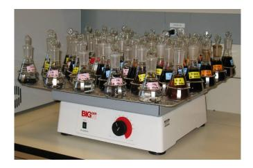
Preloading of Activated Carbon: The preloading of activated carbon for kinetics and isotherm experiments was done with 1g/L of humic acid solution prepared in deionized (DI) water. A 10% sodium azide was added to the humic acid stock solution to avoid biological growth. All the samples were equilibrated for 48 hours at 150 rpm on a rotary shaker to ensure thorough mixing. Preloaded samples having activated carbon
