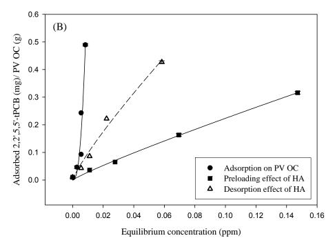
Figure 3.5 A-B: Freundlich adsorption isotherms for adsorption of tetrachlorobiphenyl in presence and absence of humic acid (A) 2, 2', 5, 5'- tPCB adsorption on CETCO organoclay (B) 2, 2', 5, 5'- tPCB adsorption on Polymer ventures organoclay
