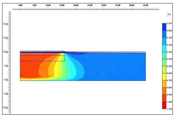
Figure 7.3-14. Volumetric strain under the coupled model.
