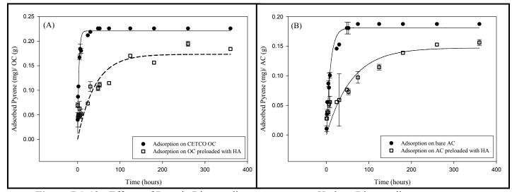
**Figure 7.1-19**. Effects of Passaic River sediment pore water, Hudson River sediment pore water, humic acid, fulvic acid and natural organic matter on the adsorption kinetics of pyrene by (A) organoclay and (B) activated carbon.
