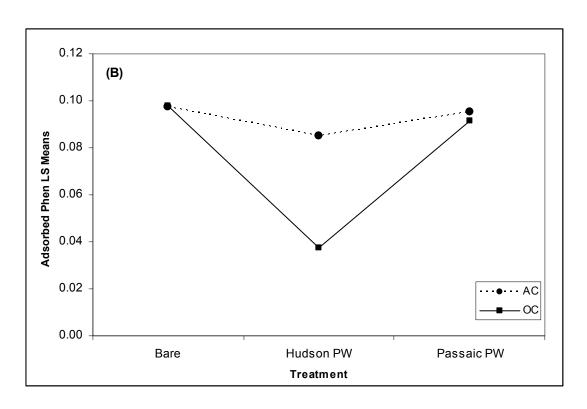
Figure 5.4B: Statistical analysis of performance of sorbents: phenanthrene adsorption on AC and OC in presence of extracted pore water (AC = activated carbon; OC = organoclay)
