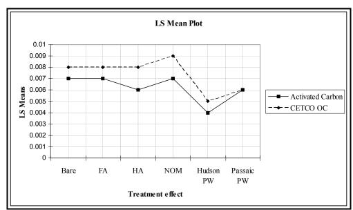
**Figure 7.1-16**. Least square mean plot to compare the effects of Passaic River sediment pore water, Hudson River sediment pore water, humic acid, fulvic acid and natural organic matter on the adsorption of 2,2',5,5'-tetrachlorobiphenyl by organoclay and activated carbon.
