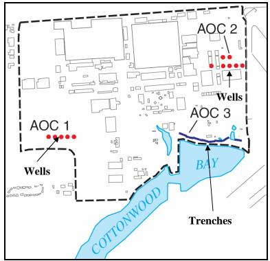
**Figure 7.2-5.** Locations of remedial wells and trenches at the Cottonwood Bay site (modified from Barker and Braun 2000).
