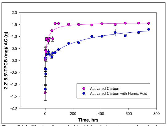
Figure 7.1-2. Kinetics of tetrapolychlorobiphenyl adsorption on activated carbon.
