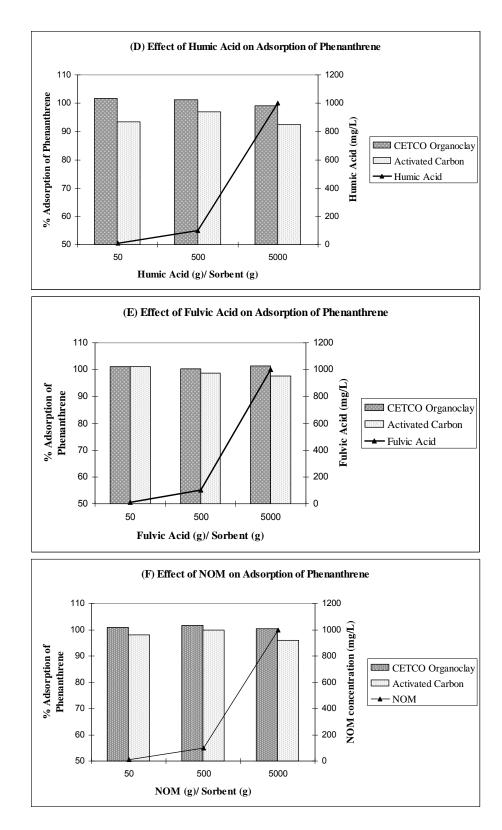
Figure 5.7D-F: Comparison of performance of organoclay and activated carbon for adsorption of phenanthrene in the presence of humic acid, fulvic acid and natural organic matter normalized to adsorption on bare materials.
