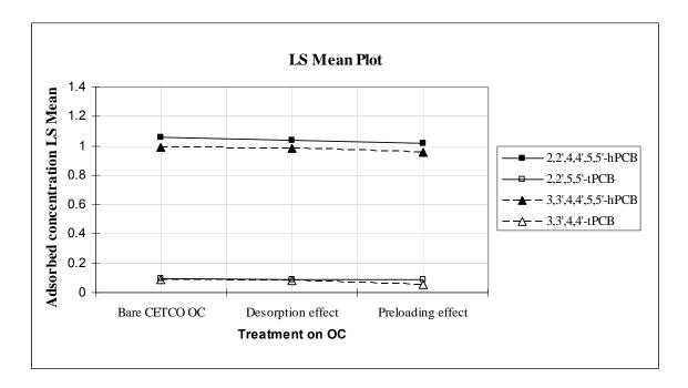
Figure 3.7: Least square means plot for adsorption of tetra- and hexa- chlorinated congeners on CETCO organoclay
