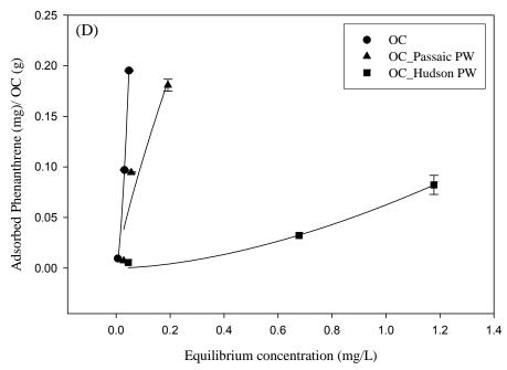
Figure 5.3 D: Adsorption contaminants in presence of extracted pore water (C) Phenanthrene adsorption on AC: Phenanthrene adsorption on OC (OC = Organoclay and PW = Pore water)
