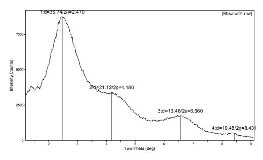
Figure 3.1.3: 2d SAXS scan for determination of d-spacing
