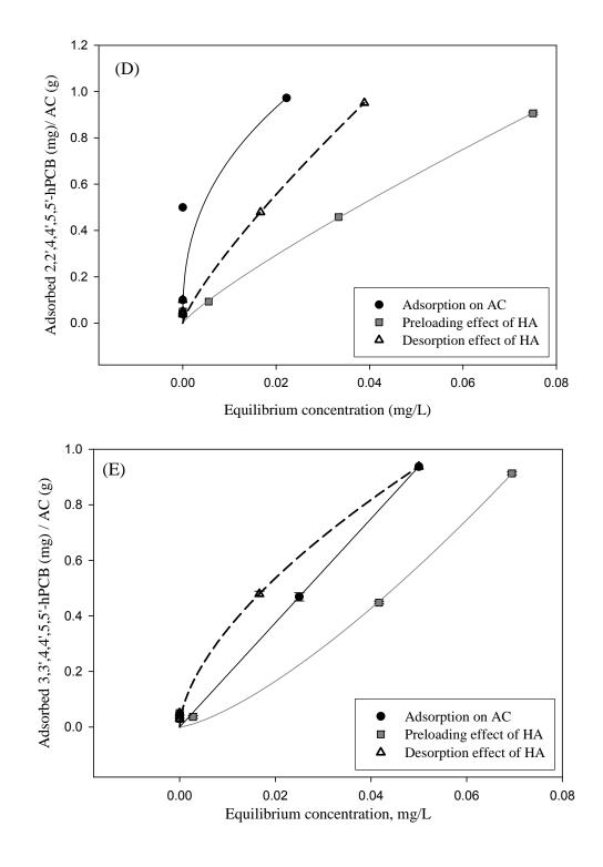
Figure 2.4 D - E. Freundlich Adsorption Isotherms for selected PCB congeners with bare AC and preloading and desorption effect of HA: (D) 2,2',4,4',5,5'-hPCB (E) 3,3',4,4',5,5'-hPCB
