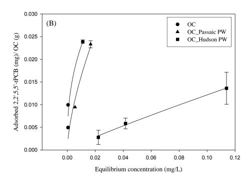
Figure 5.3 B: Adsorption contaminants in presence of extracted pore water: 2, 2', 5, 5'-tPCB adsorption on OC (OC = Organoclay and PW = Pore water)
