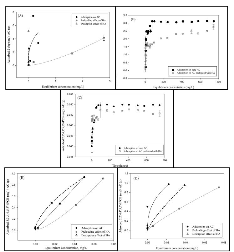
**Figure 7.1-2**. Freundlich adsorption isotherms for PCBs on bare activated carbon including preloading and desorption effects of humic acid: (A) 2-cbp, (B) 2,2',5,5'-tPCB (C) 3,3',4,4'-tPCB (D) 2,2',4,4',5,5'-hPCB and (E) 3,3',4,4',5,5'-hPCB.
