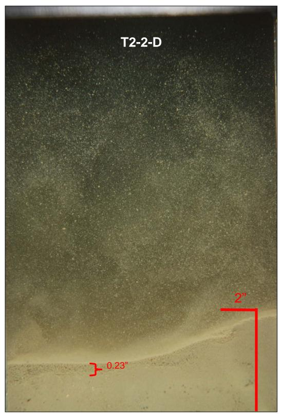
**Figure D-6**. Sediment profile image of prototype mat system area T2 (single mat with sand cap) taken in capping material.
