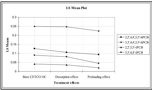
**Figure 7.1-12**. Least square mean plot to determine the effects of different humic acid treatments on the performance of CETCO organoclay in sequestering tetra- and hexa-chlorobiphenyls.
