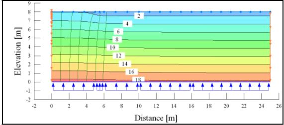
**Figure C-9**. Pressure head contours (m) and flow paths ( $k_{GT} = 0.001 \text{ x } k_{SED}$ ).
