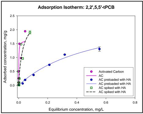
**Figure 7.1-9.** Adsorption isotherm of 2,2',5,5'-tetrachlorobiphenyl onto activated carbon.
