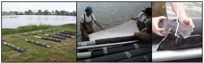
**Figure 6.3-2**. Small-scale geotextile test mat deployment.
