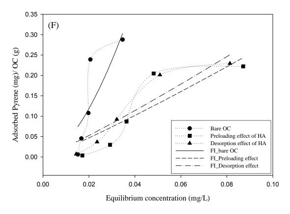
Figure 4.2 F: Pyrene adsorption on organoclay
