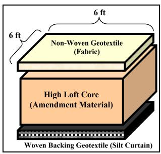
Figure 6.3-1. Construction diagram of small-scale geotextile test mats.
