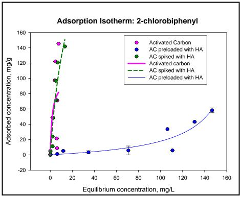
**Figure 7.1-8.** Adsorption isotherm of 2-chlorobiphenyl onto activated carbon.
