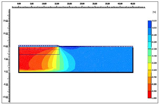
**Figure 7.3-9**. Volumetric strain after 95% consolidation under the uncoupled consolidation model.
