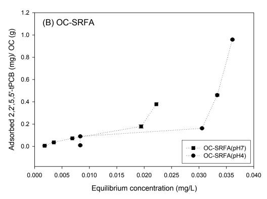
Adsorption of 2, 2', 5, 5'-tPCB in presence of Suwannee River FA at pH 4 and 7 (A) Activated carbon (B) Organoclay
