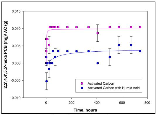
**Figure 7.1-3.** Kinetics of hexachlorobiphenyl adsorption on activated carbon.
