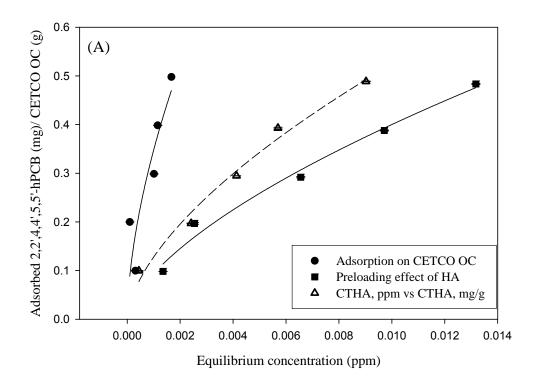
Figure 3.6 A: Freundlich adsorption isotherms for adsorption of hexachlorobiphenyl on CETCO organoclay in presence and absence of humic acid: 2, 2', 4, 4', 5, 5'-hPCB
