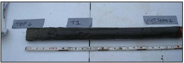
Figure I-2. Sediment core collected from treatment area T1 (mat only).
