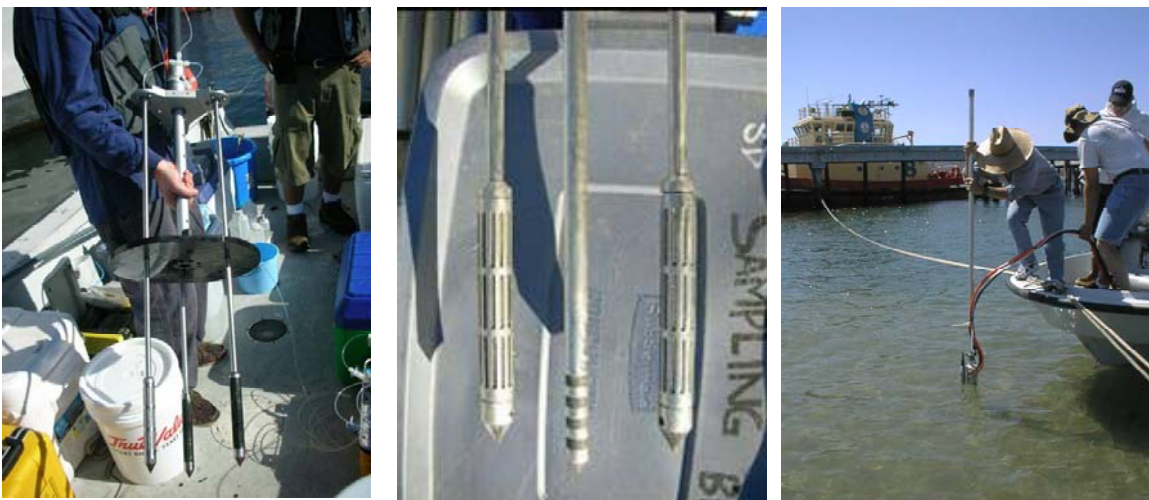
Figure 4-1. Photos of Trident Probe during November sampling event, illustrating use of multiple pore water sampling probes and sand packs to increase flow rate in finer grained sediments.
