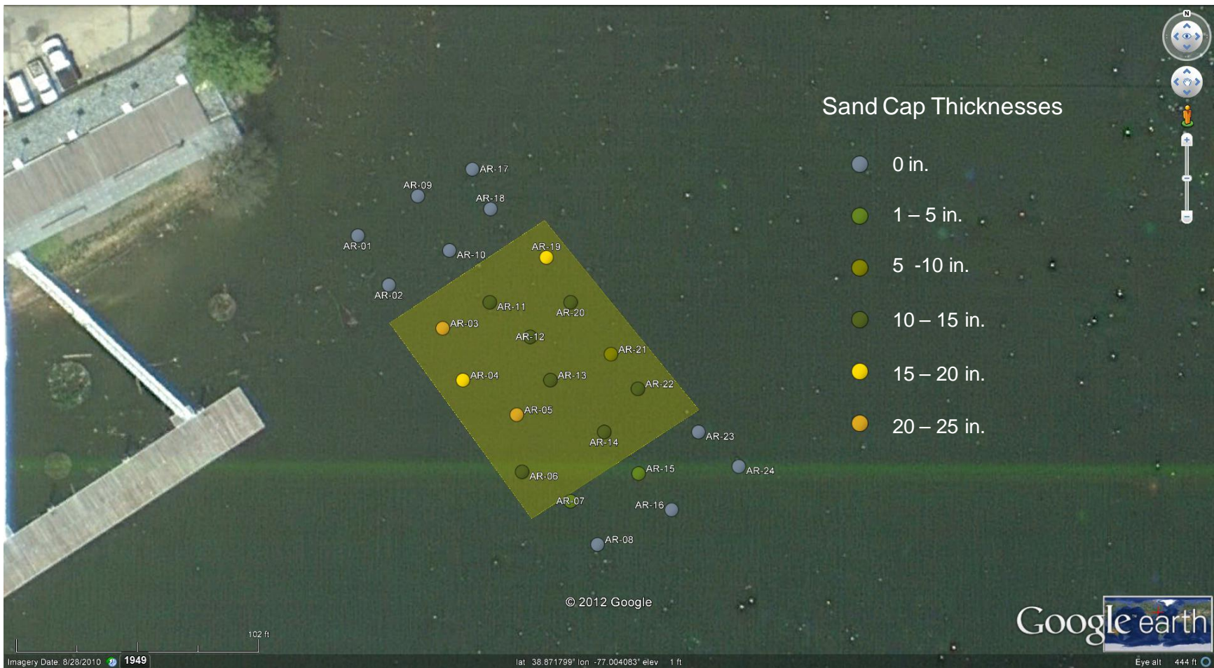
Figure 10. SED-FSP grain size measurements for Anacostia River sand cap survey.
