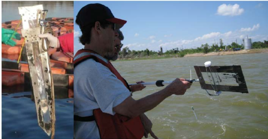
Devices that expose flat sheets of absorptive materials (POM or PE)
