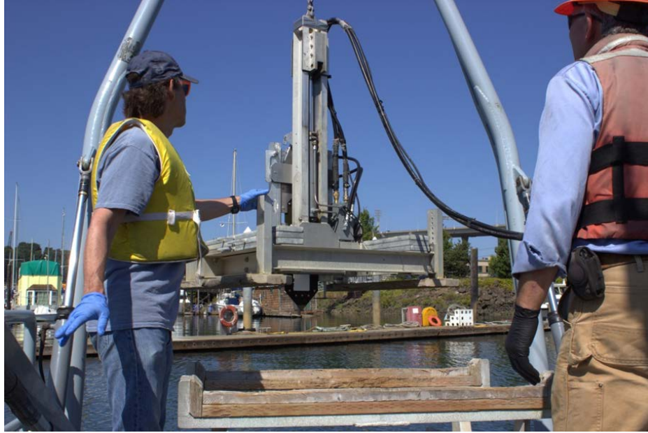
Image 4. Passive Samplers Deployed in the Field from Boat
