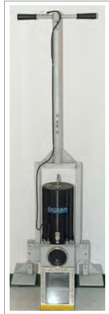
C. Longer handle for hand deployment in small boat in water depths to 6 feet.
