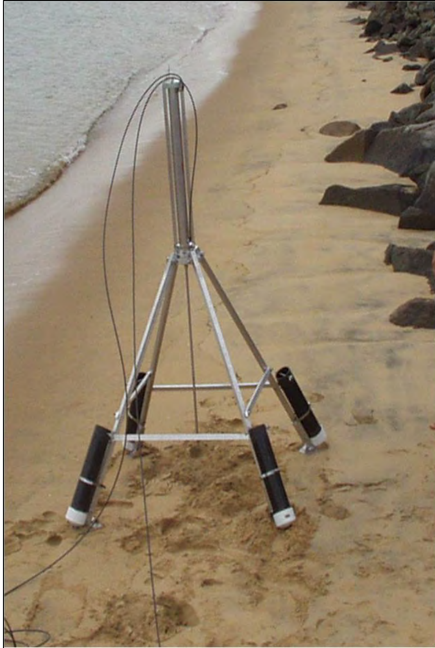
Figure 25. SED-FSP system; probe and frame assembly.
