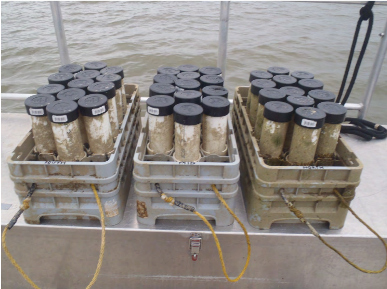
Figure 27. Sediment traps used during the 2014 and 2016 sampling events. Black caps were removed after deployment and replaced prior to retrieval.
