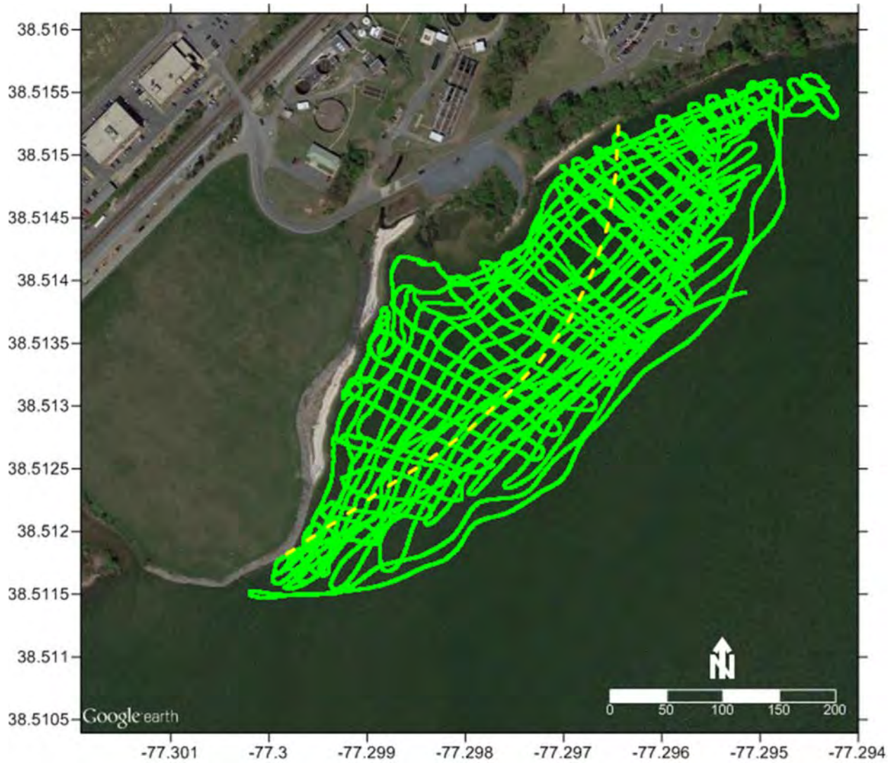
Figure 16. Typical track line for the bathymetric surveys at Quantico Embayment. This track is from the 2015 post-cap survey.
