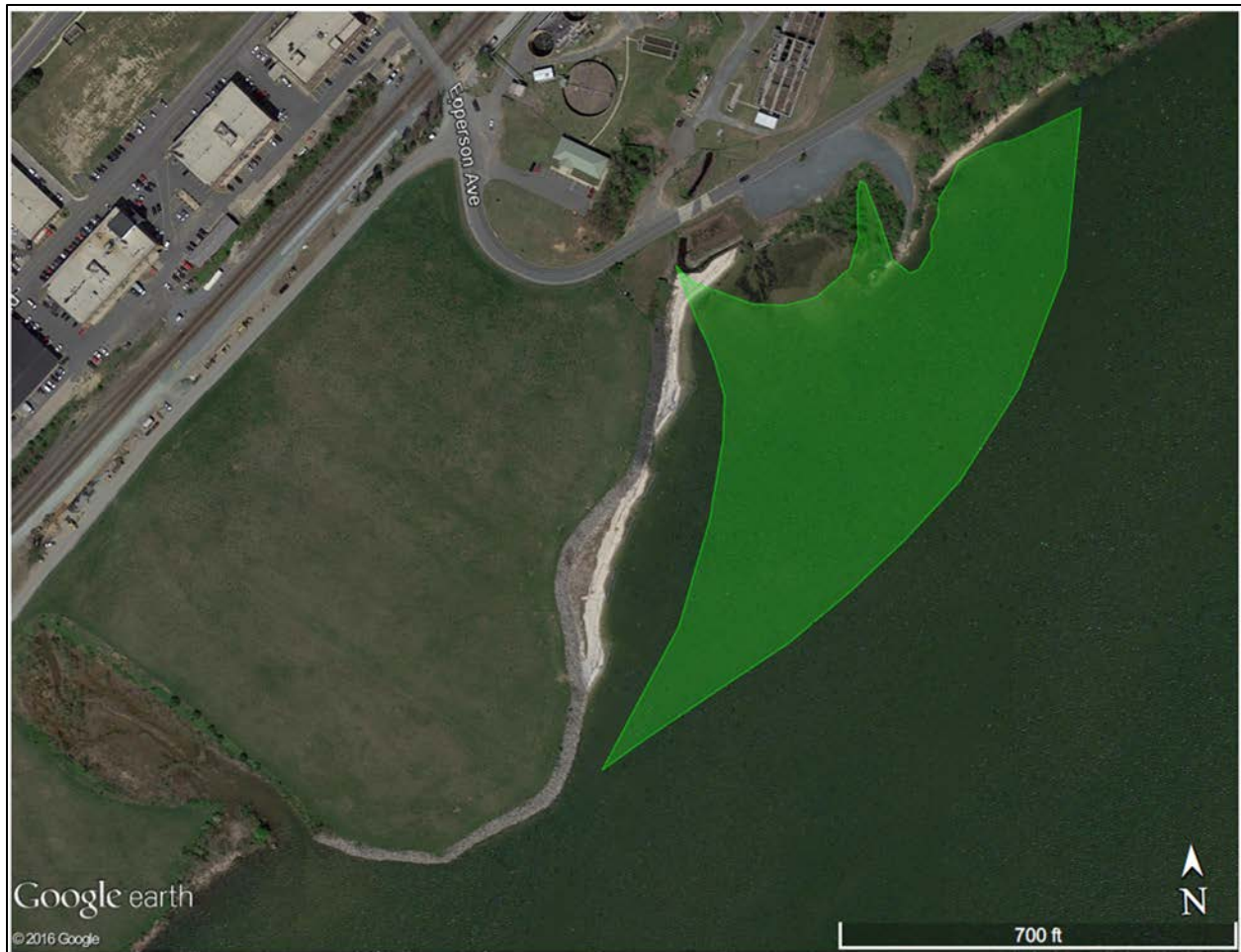
Figure 9. Approximate extent of TLC in the Quantico Embayment. The cap area encompasses sediment with surface sediment DDX concentrations greater than or equal to 200 \mu\text{g}/\text{kg} (Adapted from Battelle 2008).
