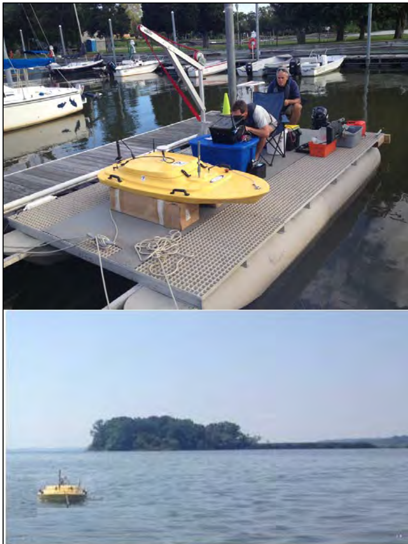
Figure 15. Teledyne Oceanscience Z-Boat 1800 remote control hydrographic survey boat used during the 2015 and 2016 surveys undergoing preparation (top photo) and surveying in work area with Chopawamsic Island in the background (bottom photo).
