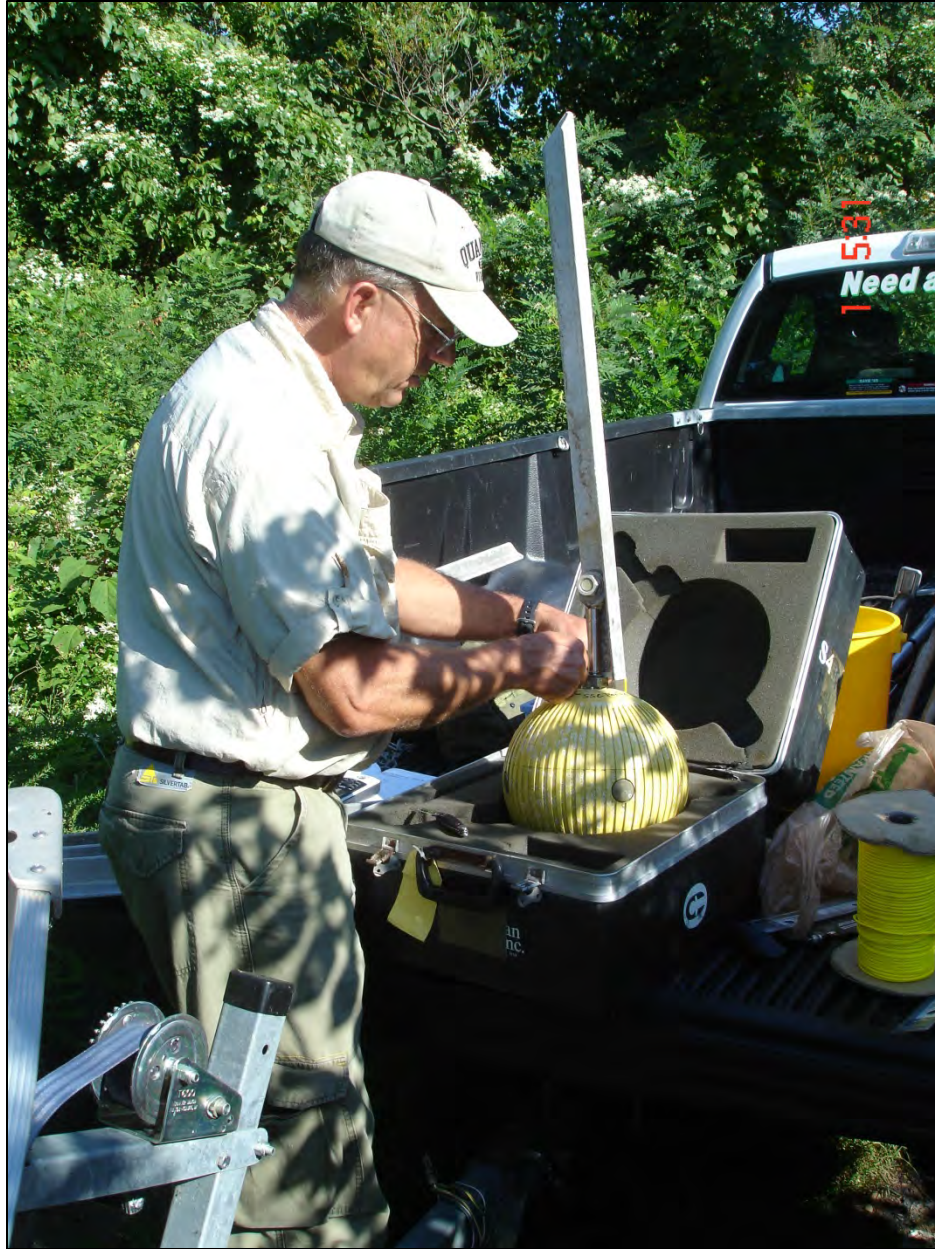
Figure 20. Preparing the aluminum angle iron spike to support the S4 current meter.
