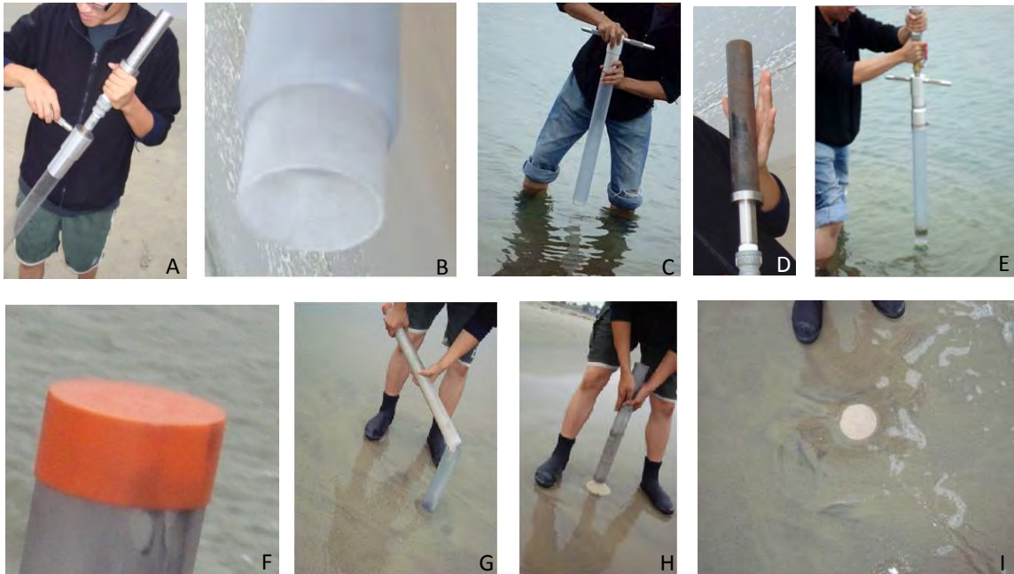
Figure 2. Field sampling procedure for the iCorer including (A) install the handles, (B) liner protruding from sleeve, (C) initial hand push, (D) slide hammer installation, (E) slide hammering, (F) install the cap on top and remove the liner, (G) pour the replacement material, (H) remove the outer sleeve, and (I) the completed core location with replacement material installed.
