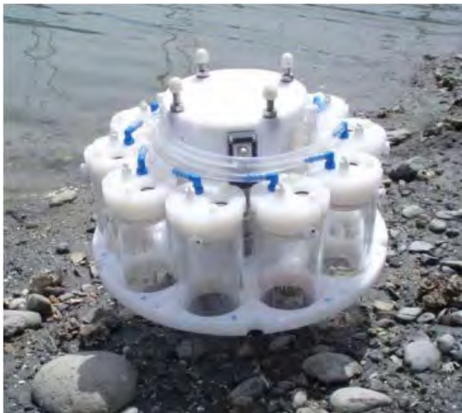
Figure 32. Second Generation SEA Ring Device utilized for assessment of in situ bioaccumulation.
