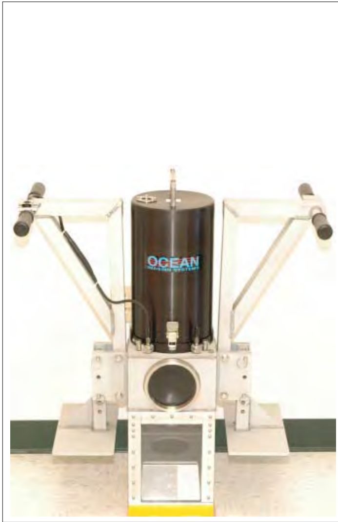
A. Hand held version for shallow stream and inter-tidal work, deployed by walking. Weight is approximately 40 lbs.
