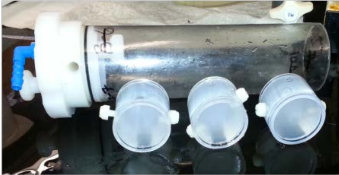
Figure 5-9. Embryo drums used for housing mussel embryos within exposure chambers in the SEA Ring for in situ exposures.
