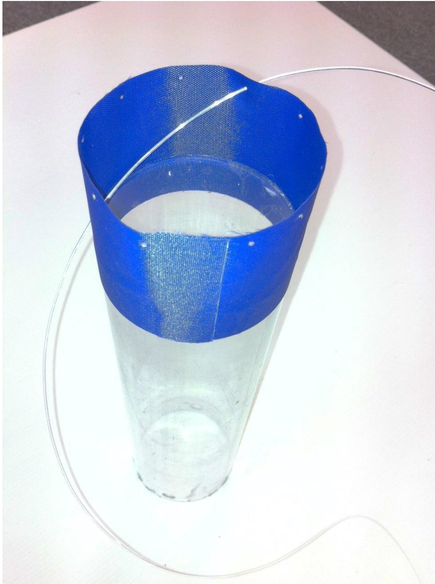
Photo 2: Threading the core catcher line
