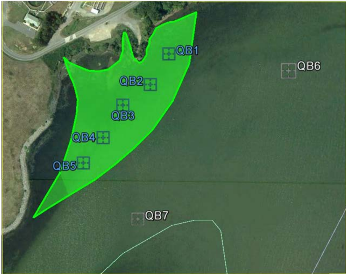
Figure 5-7. Sampling locations for MCB Quantico site. The area in green represents where a thin-layer sand cap was installed in April 2014. Cap area encompasses sediment with surface sediment DDX concentrations greater than or equal to 200 \mu\text{g}/\text{kg} .
