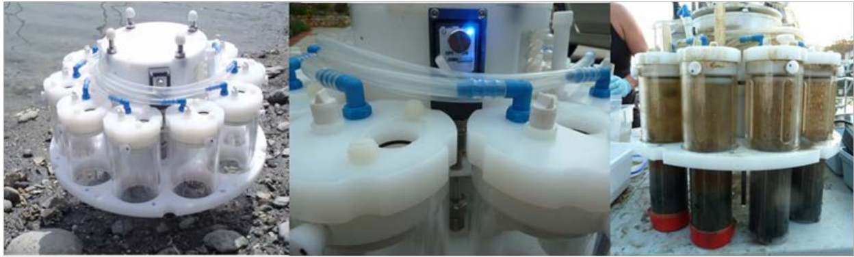
Figure 5-1. SEA Ring platform for conducting in situ toxicity and/or bioaccumulation experiments.
