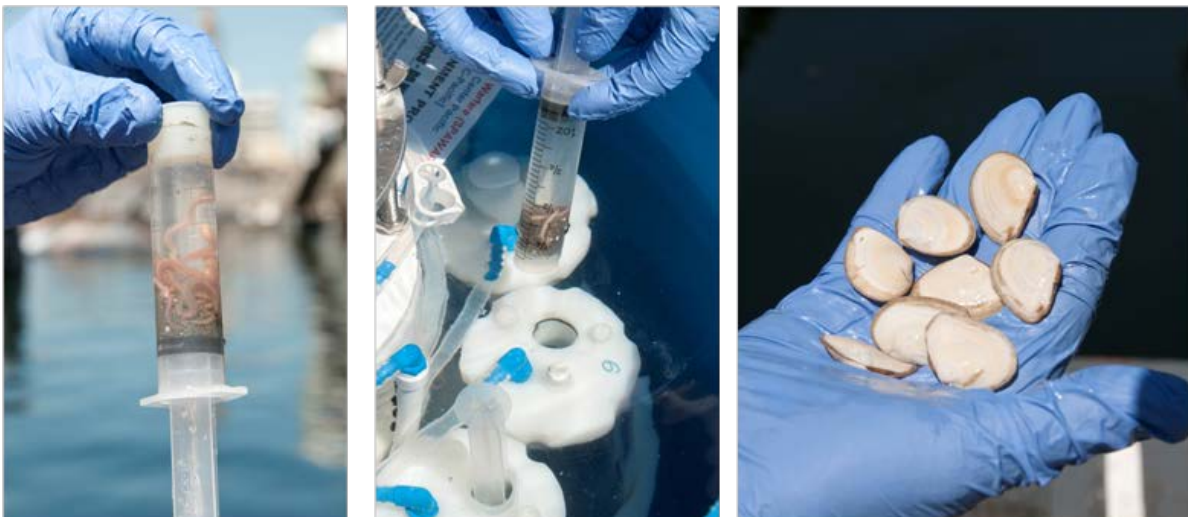
Figure 2-3. Smaller organisms (e.g., polychaetes and amphipods) are delivered by pre-loaded syringes while larger organisms (e.g., clams) are placed into chambers prior to deployment.
