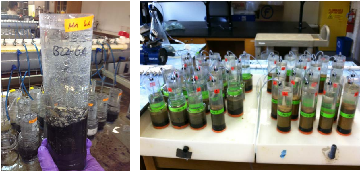
Figure 5-5. Intact sediment cores collected for flow-through (left) or static-renewal (right) ex situ bioassays, as well as sampling for sediment chemistry and benthic community analyses.
