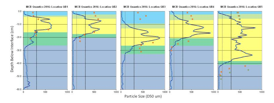
Figure 7. Examples of SED-FSP Profiles for the Multi-metric Stations QE1–QE5 (left to right) during the 2016 Post-cap Survey. Blue lines and diamonds represent the SED-FSP data, while orange square symbols (and green for QE5 station duplicate) show measured D50s from the cores collected at these stations. Blue colors indicate native material, green tones indicate mixed zones, and yellow color indicates predominant sand.
