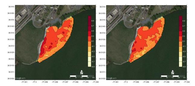
Figure 6. Difference Map for the 2014 Pre-cap Baseline Compared to the 2015 Post-Cap Survey (left) and Difference Map for the 2014 Pre-cap Baseline Compared to the 2016 Post-cap Survey (right). The yellow dashed line indicates the offshore boundary of the area targeted for the thin-layer cap. Positive differences indicate 2015 elevations that are higher than 2014 elevations. Units are meters.
