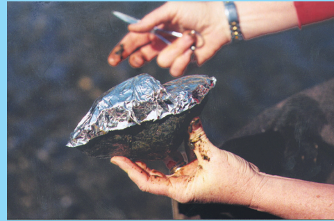
b. Top-rock scrape method: scraped area of a cobble covered with foil to determine the area sampled.
