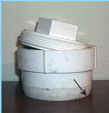
c. Gravel sampler: beveled edge (arrow) on bottom of sampler improves coring into gravel substrates.
