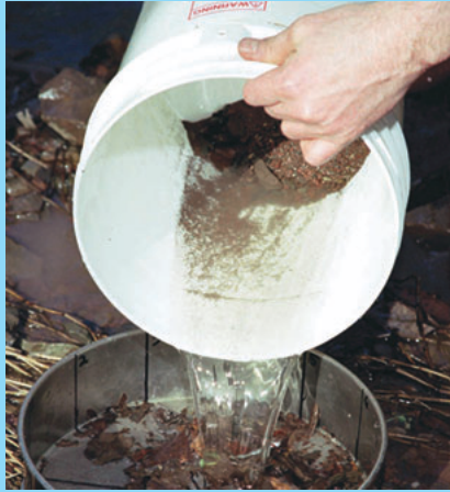
f. Elutriating the discrete collection using a bucket and sieve.
