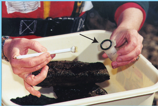
a. SG-92 sampler: preparing to scrape a cobble with microalgal periphyton brush (arrow points to O-ring seal on bottom of SG-92).
