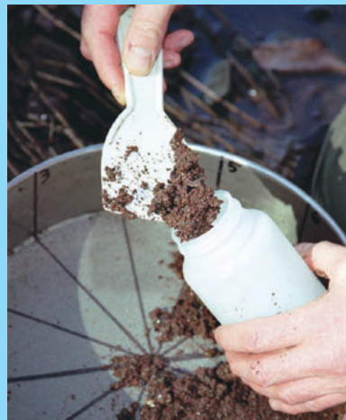
k. Placing the main-body sample component into a standard sample bottle.
