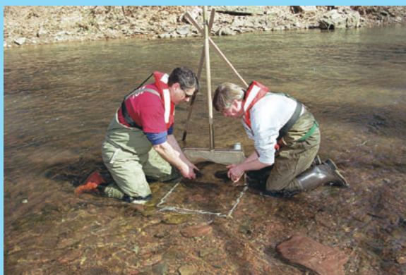
a. Two crewmembers taking a discrete collection using Slack sampler.
