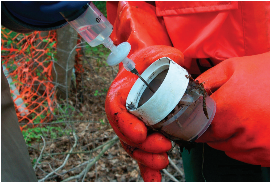
Figure 7. Collecting a field sample from nylon-screen diffusion sampler by using syringe, filter, and hypodermic.
