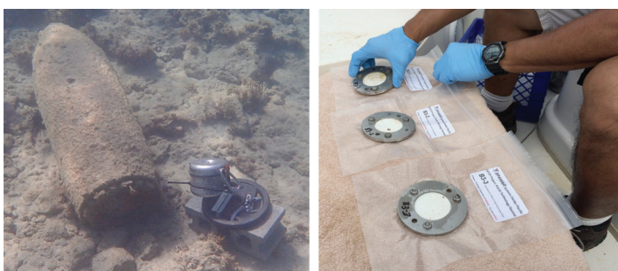
Figure 8. POCIS Deployment: (a) Placement of a POCIS Canister Adjacent to a Munition and (b) Preparing POCIS Samplers for Laboratory Analysis Following Recovery from Field (Courtesy of Rosen et al., 2017)
