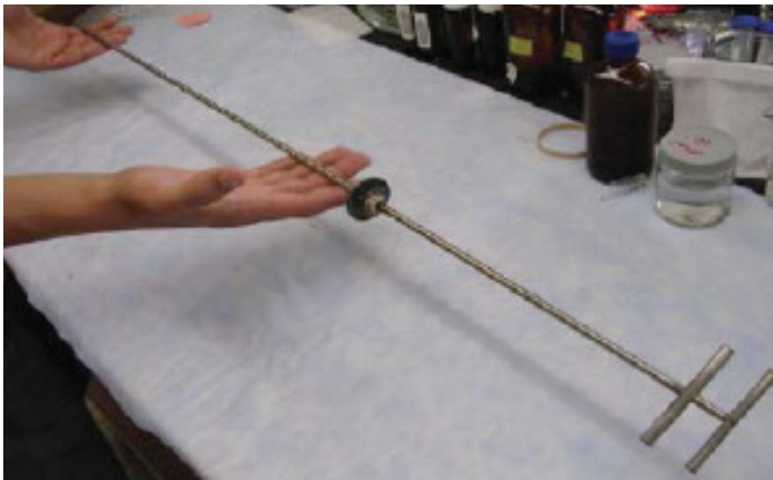
Figure 7. SPME Enclosed in a Metal Probe for Insertion into the Sediment (Courtesy of Menzie et al., 2016)
