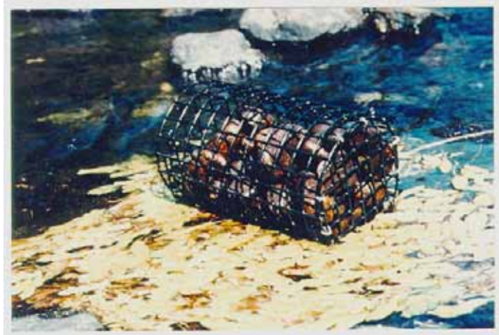
FIGURE 6-1. Rock-filled wire basket used as introduced substrate.
