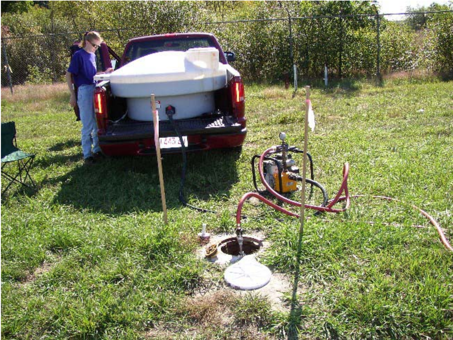
Figure 2-4. Reagent Mixing and Injection System
