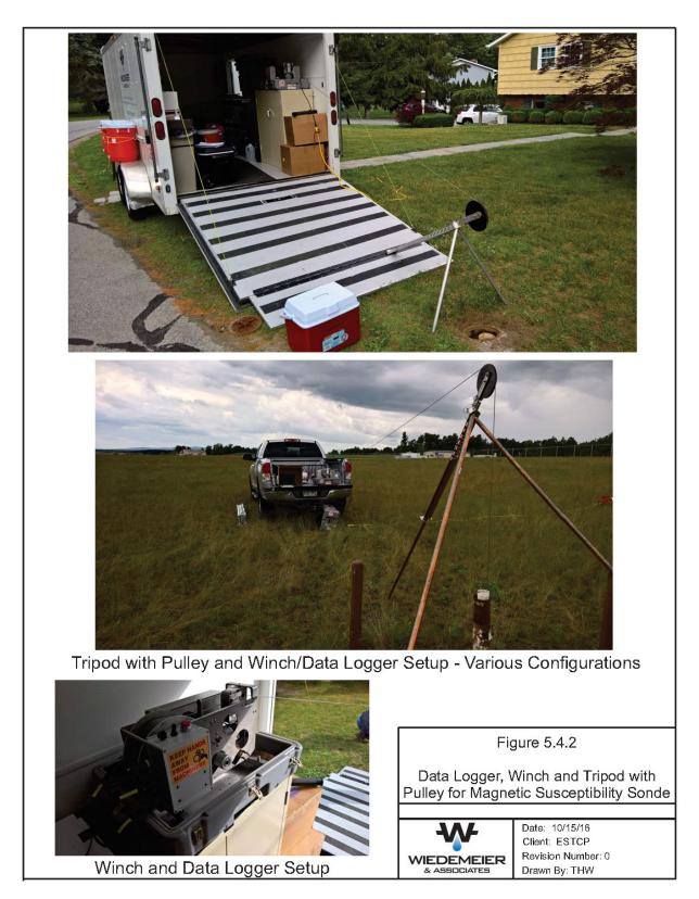
Figure 5.4.2. Data Logger, Winch and Tripod with Pulley for Magnetic Susceptibility Sonde
