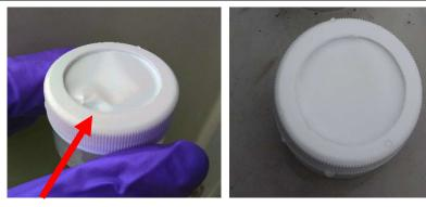
A wrinkle in the peeper membrane due to damage or mishandling; do not use the peeper for field deployment, although it can be used as a Trip Blank if needed
