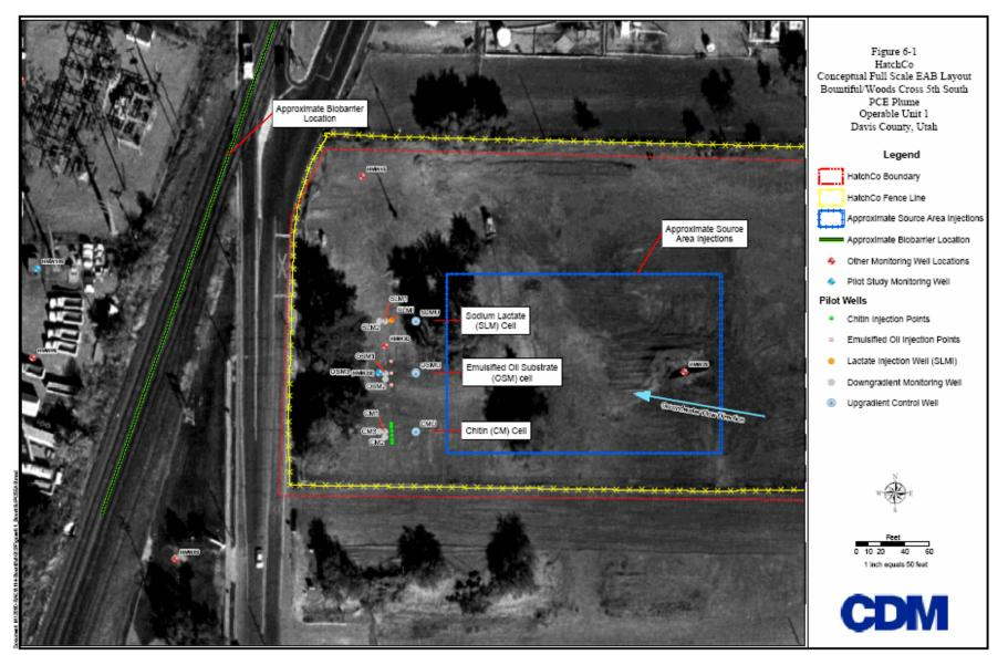
Figure 6-1.—Conceptual Full Scale EAB Layout
