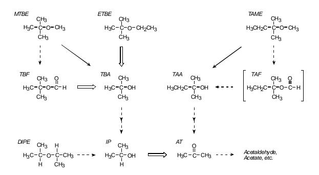
Figure 1. Proposed Degradation Pathway of MTBE by Bacterial strain PM1 (Church and Tratnyek, 2000)
