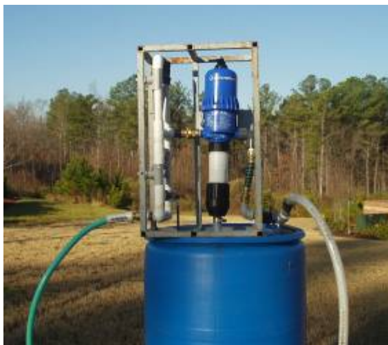
Figure 5.8 Setup of Automatic Metering System for Dilution of Concentrated Emulsion Product (Photo courtesy of EOS Remediation, Inc.)
