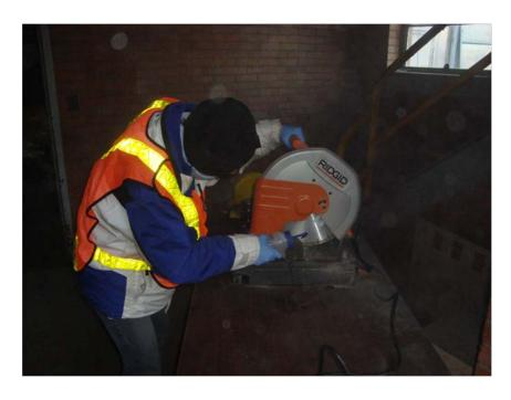
Figure 2 – Photograph of the cutting of the 1 cm thick discs from the recollected rock core at the NAWC site.
