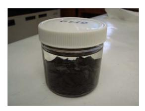
Figure 5 – Photograph of the 125mL jar containing the TCE extract from grey mudstone.
