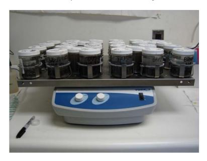
Figure 6 – Photograph of the orbital shaker where the TCE and PCE extracts remained for 24 hours to attain complete extraction of VOCs.
