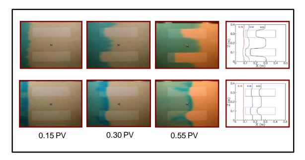
Figure 1. Sweeping efficiency comparison during lab-scale testing.
