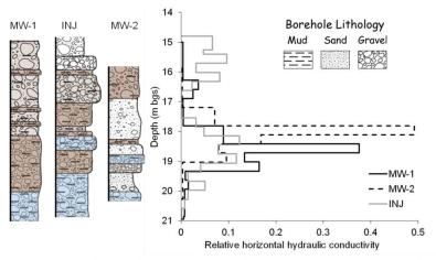
Figure 9. Borehole geologic log in well screen interval and EBF data interpreted as the vertical distribution of relative horizontal hydraulic conductivity at each individual well. Borehole log brown shading indicates silt content with darker zones showing more silt. Borehole log blue shading indicates zones of more consolidated materials.
