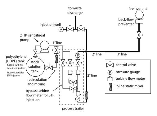
Figure 15. Schematic of the process and injection equipment for the baseline and STF injections.
