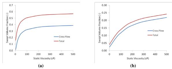
Figure 13. Results of simulations examining the relation between viscosity and improved distribution to low-k layers.
