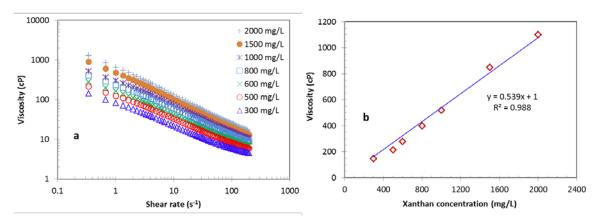
**Figure 11. Xanthan gum concentration influence on fluid viscosity and rheology.** (a) Viscosity as a function of shear rate, and (b) Viscosity at low shear rate (0.3 s<sup>-1</sup>) for several xanthan concentrations. All solutions were made in DI water.
