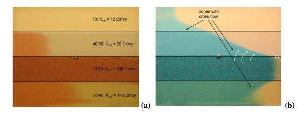
Figure 3. Fluid distribution in flow cell experiments after injection of 0.67 PV.
