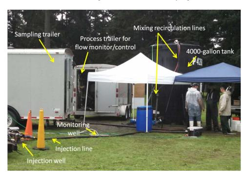
Figure 14. Injection and monitoring equipment layout.
