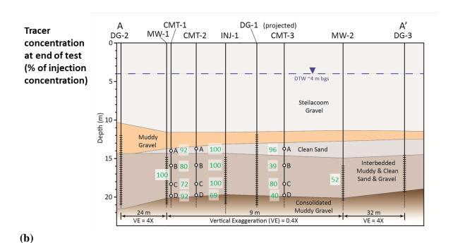
Figure 19. Cross-section of treatment zone with tracer distribution during baseline injection test.
