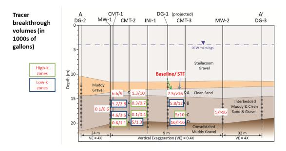
Figure 20. Cross-section of treatment zone with tracer distribution during baseline injection test versus STF injection test.
