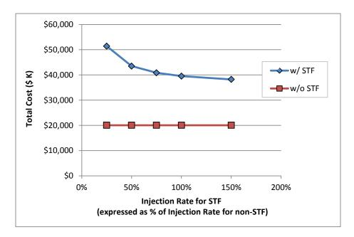
Figure 23. Sensitivity of cost of shear-thinning technology to injection rate.
