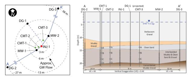
Figure 8. Layout of treatment cell.
