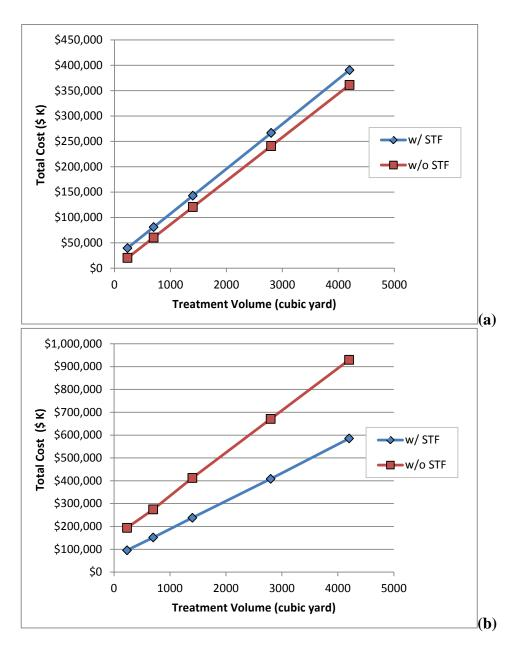
Figure 25. Sensitivity of cost of shear-thinning technology to volume of treatment zone.
