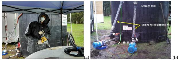
**Figure 16. Preparation of the xanthan stock solution.**a) initial mixing and b) continued hydration with additional recirculation mixing in the storage tank.
