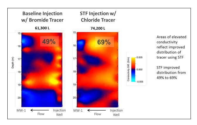
Figure 21. Comparison of amendment distribution using the ERT images.
