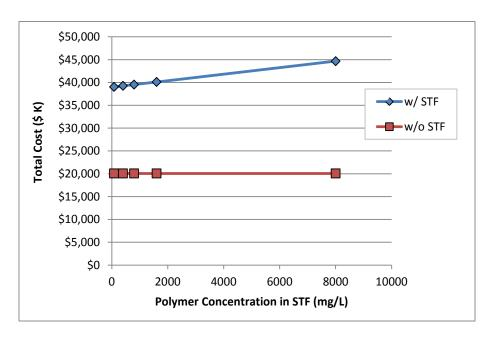
Figure 24. Sensitivity of cost of shear-thinning technology to polymer concentration. (Scenario 1: single injection)
