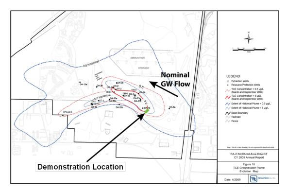
Figure 7. TCE groundwater plume evolution at Area D.
