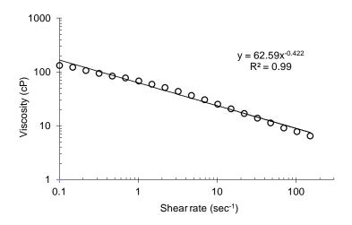
Figure 18. Rheology of STF injection solution used in the field demonstration. The data in the power-law region have been fitted with an Ostwald-De Waele relationship according to Lopez et al. (2003).
