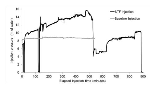
Figure 17. Injection pressure recorded during the baseline (control) and STF injection tests.
