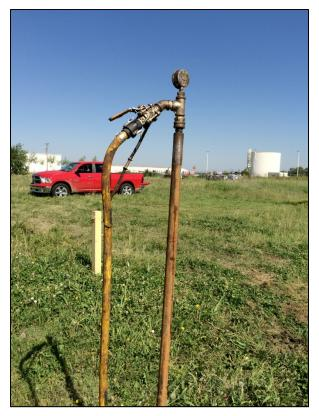
Photo 11: EHC injection rod with hose connected to injection manifold.
