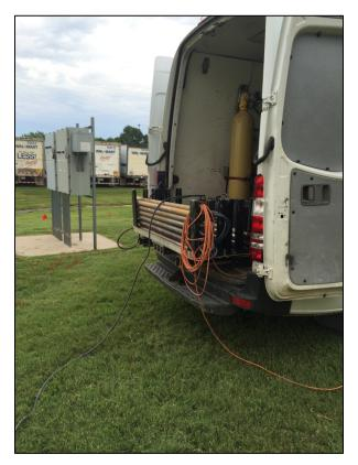
Photo 4: HPT trailer with cables in the HPT rod shown.
