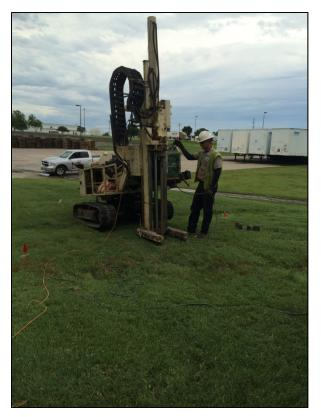
Photo 3: HPT drilling rig.
