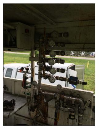
Photo 8: Injection manifold.
