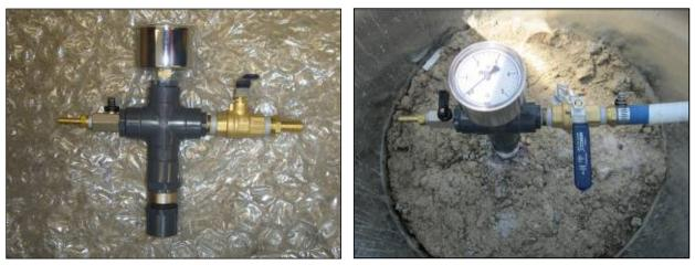
**Figure 27:** Injection wellhead design
