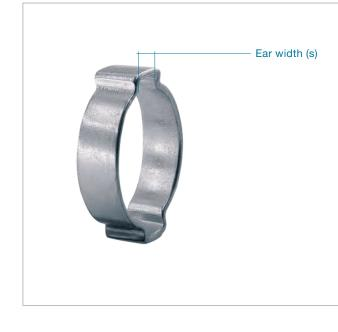
2-Ear version: extended clamping range Compact one-piece clamp: for robust, secure connections Clamp ear: fast and simple installation, visible deformation provides evidence of proper closure Deburred edges: reduced risk of damage to parts being clamped
