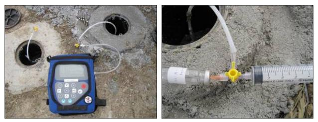
Figure 21: GEM2000 readings and vapor sampling
