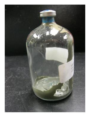
Figure 2-2: Microcosm Bottle with Soil at 30 Percent Moisture
