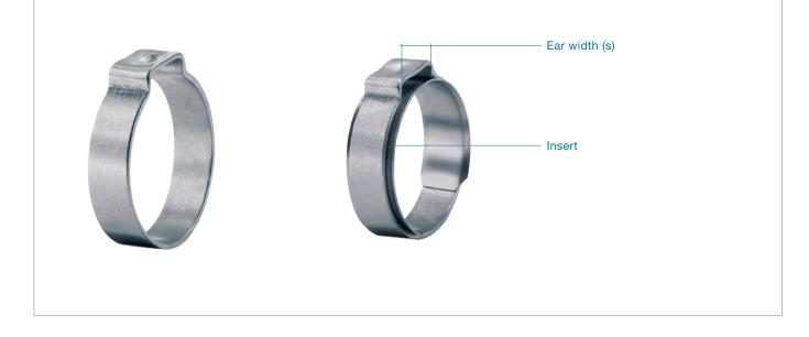
Compact one-piece clamp: for robust, secure connections, miniature sizes Clamp ear: fast and simple installation, visible deformation provides evidence of proper closure Deburred edges: reduced risk of damage to parts being clamped With insert Pre-shaped insert: effective and powerful all-round seal
