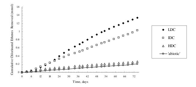
Figure 2-1. Enhanced Chlorinated Ethene Removal from NAPL in Column Studies (Cope and Hughes 2001).
