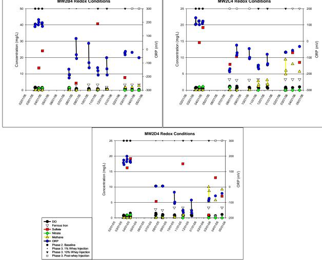
Figure 4-7. Trends in Treatment Cell 2 Port 4 Redox Conditions During Demonstration.
