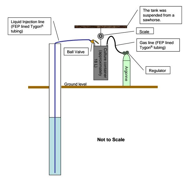
Figure A-1. Schematic of culture injection system.
