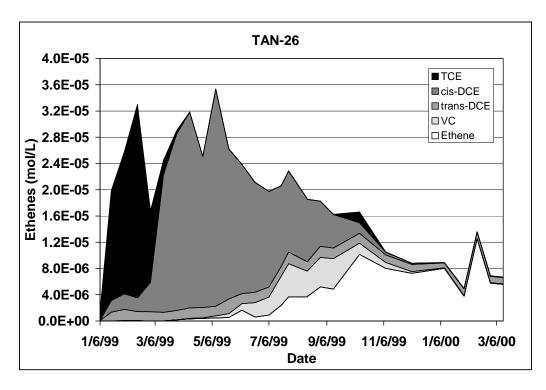
Figure 2-2. Enhanced Mass Transfer and Bioavailability of TCE Through Sodium Lactate Addition.
