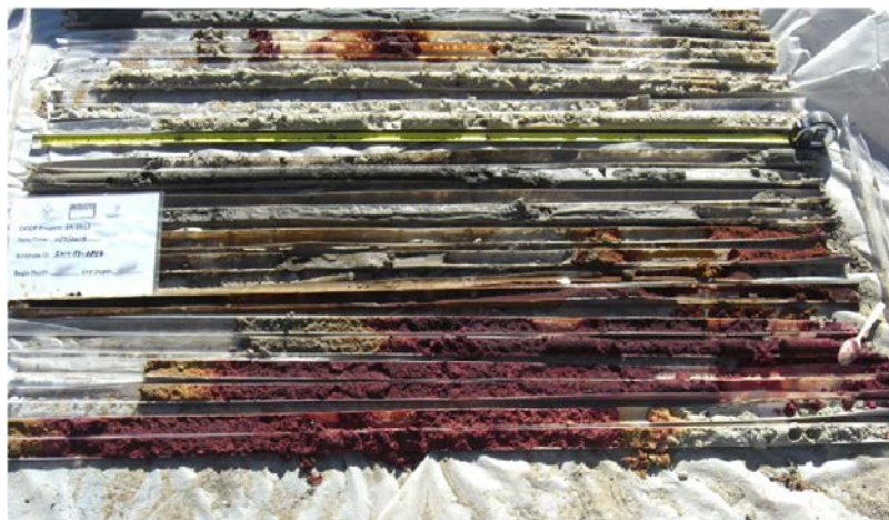
Figure 5-18. Sediment cores used to vertically characterize the presence/absence of permanganate within the control plot.
