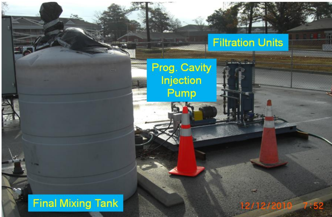
Figure 5-15. Fluid injection and filtering system.
