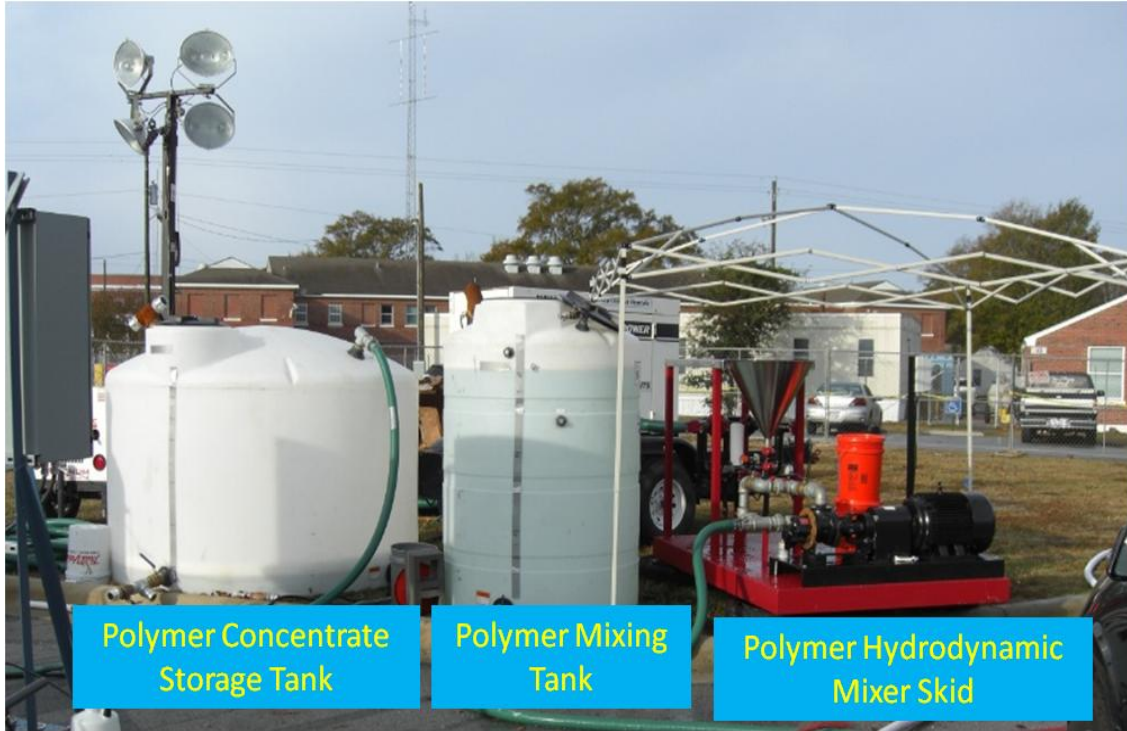
Figure 5-13. Xanthan gum/SHMP mixing system.
