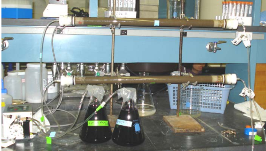
Figure 10. 1-D packed columns for evaluation of permanganate and SHMP transport through site porous media. The top column is permanganate-only and the bottom is permanganate + SHMP.
