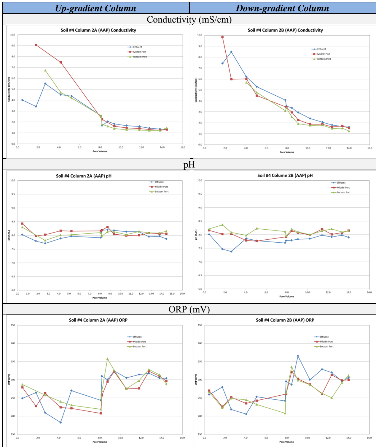
Figure 4.3.8 Column Experiment: Soil #4 with AAP Treatment – Geochemical variation with increasing groundwater PV.
