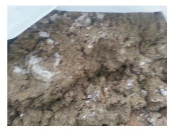
Material mixed with LKD approximately 2 hours after mixing  $% \left( 1\right) =\left( 1\right) +\left( 1\right)$
