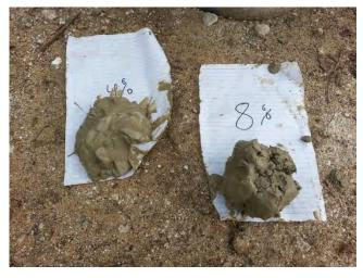
Results of the LKD bucket test after 96 hours (conducted on Friday 10/9/15). 4% by volume is still soft. 8% by volume is workable material.
