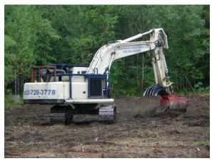
Tree mulcher regrinds tree shreddings into topsoil
