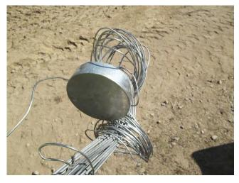
Stainless steel well casing found wrapped around blender head
