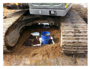
Hydraulic fluid spill from the Volvo excavator.
