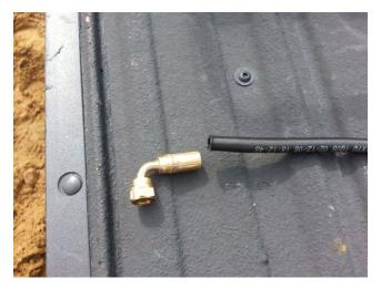
Hydraulic fitting that separated under the floor board of the excavator
