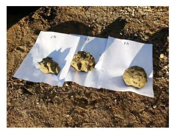
Portland cement and soil mix soil ratio results after 14 hrs. of cure time
