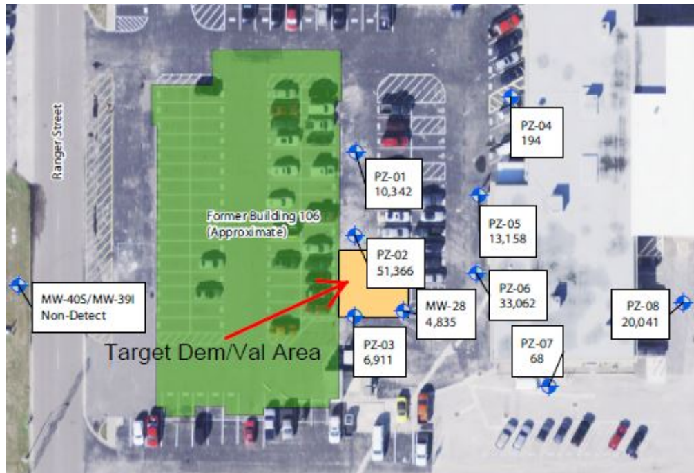
Figure 4-4. Total Chlorinated Ethenes in Select Groundwater Monitoring Wells in Shallow Sand Aquifer
