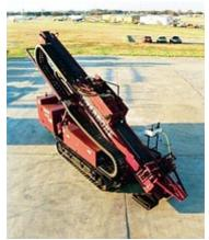
Horizontal directional drilling has been used for the installation of wells for a number of different environmental applications. Courtesy of Advanced Directional Drilling Systems.
