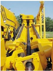
For remediation of contminant plumes, horizontal wells can offer significant advantages over vertical wells. Courtesy of Central Mine Equipment Co.
