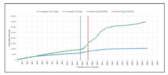
Figure 8. Contaminant Recovery Results at Building 379, NASNI, California
