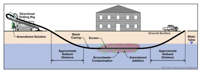
Figure 3. Surface to Surface Drilling
