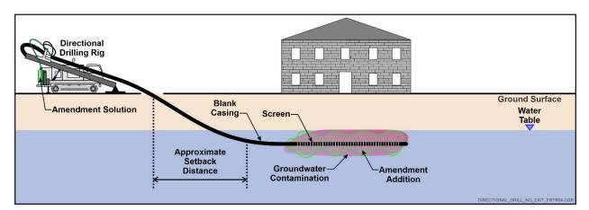
Figure 4. Blind Hole Drilling
