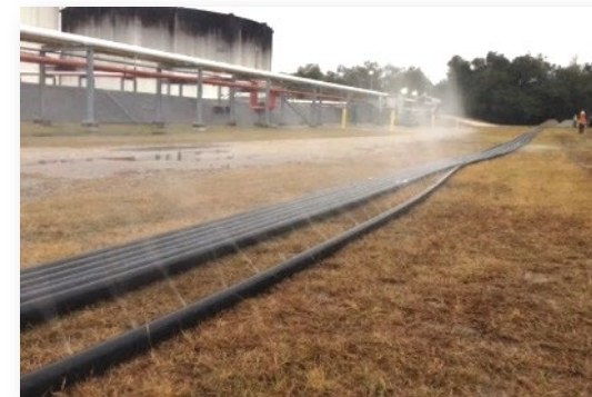
Water being pumped through horizontal air-sparge well demonstrating uniform flow through well screen (DTI 2011)
