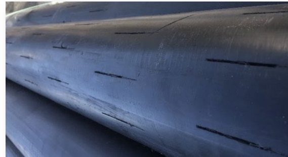
Varying well materials and custom slotting: SS (GW extraction), HDPE (injection), PVC (SVE and injection) (EDTD and DTI 2023)
