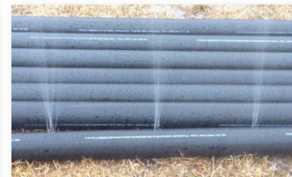
Water being pumped through horizontal air-sparge well demonstrating uniform flow through well screen (DTI 2011)
