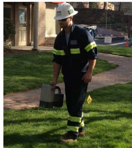
Walk-over locating technology, Falcon F2 system (EDTD and Underground Construction 2023)
