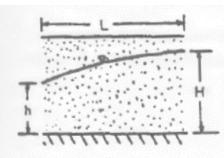
Water table flow from a line source to a drainage trench
