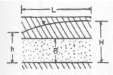
Confined flow from a line source to a drainage trench
