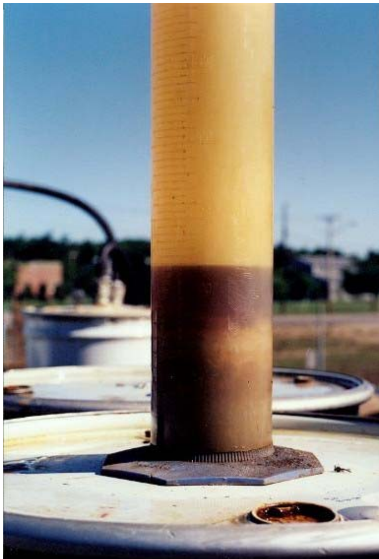
Figure 5-3. Photo of Fuel Floating Solids and Water at NCBC Davisville
