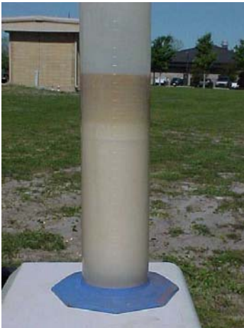
Figure 5-1. Volume Measurements Aqueous Stream with Emulsified Fuel in Water, Floating Solids and Relatively Clean Fuel
