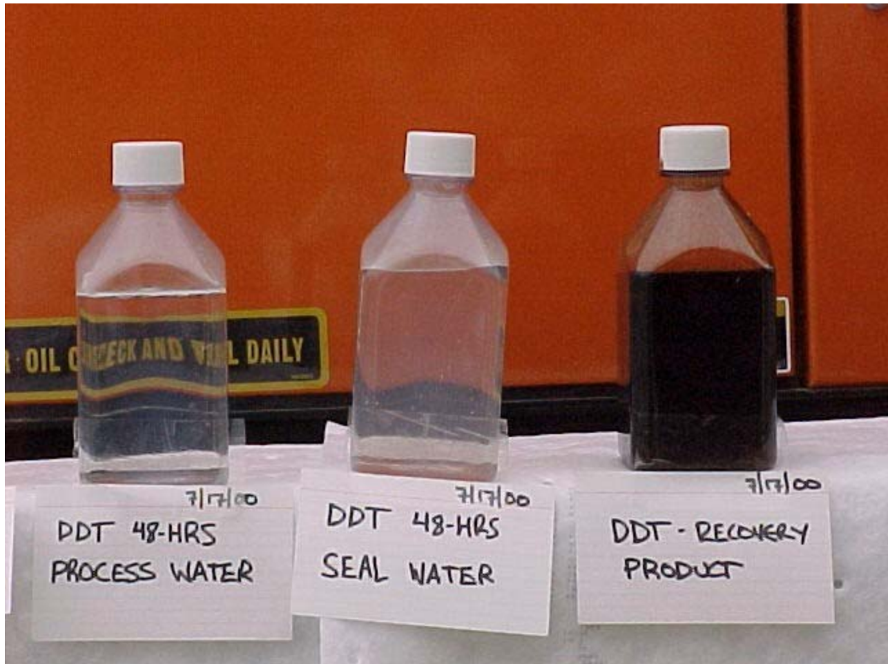
Figure 5-8. Samples Of The Process Water, Seal Water, And Free-Product Recovered During The Dual Drop Tube Test
