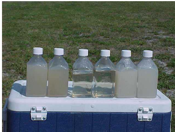
Figure 5-2. Comparison of Aqueous Streams During Knockout, Dual Drop tube and Conventional Tests (L to R)
