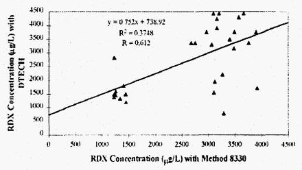
Figure 2-11: Comparison of DTECH RDX Results to Method 8330
