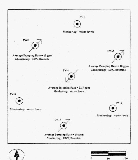
Figure 2-14: Pumping Rates and Monitoring During Tracer Test
