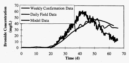
Figure 4-7: Model Predicted Breakthrough Curve at EW-3 from One-Layer Model
