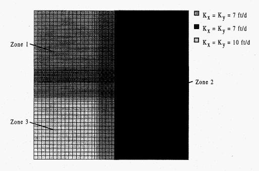
Figure 4-17: Hydraulic Conductivity Zones for Layer 2
