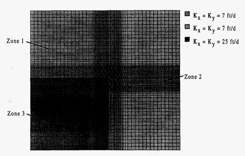
Figure 4-16: Hydraulic Conductivity Zones for Layer 1
