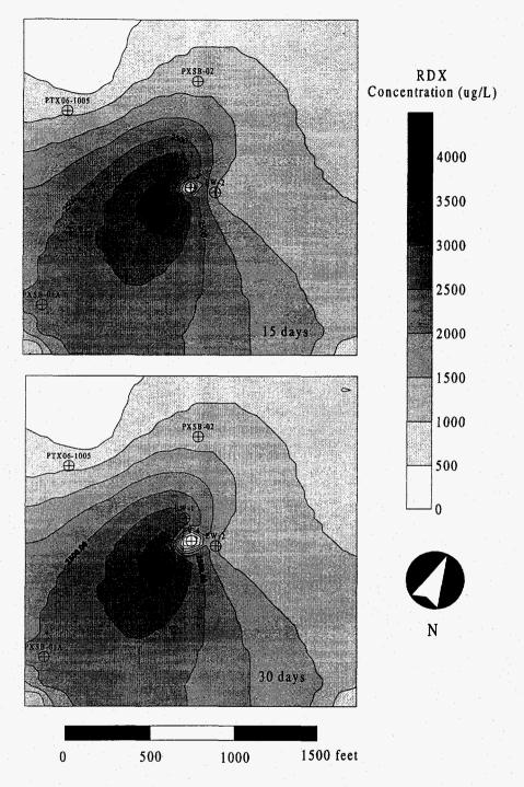
Figures 4-25 and 4-26: RDX Contours at 15 and 30 Days in the Tracer Test
