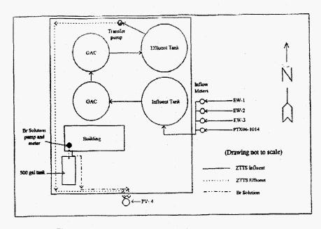
Figure 2-1: Schematic Drawing of the Site Arrangement
