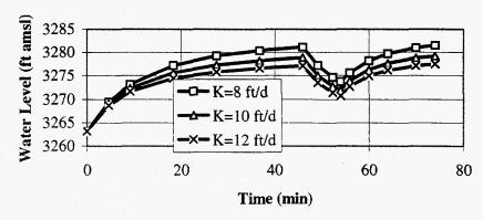
Figure 4-4: Sensitivity to Hydraulic Conductivity in Initial Injection Model at PV-4
