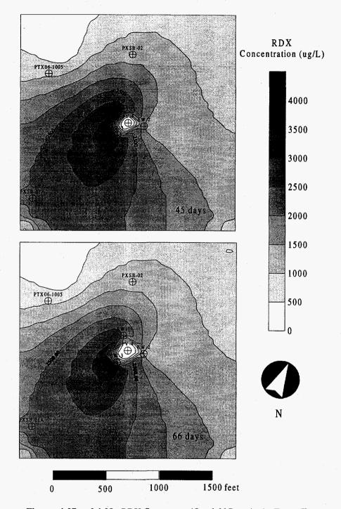
Figures 4-27 and 4-28: RDX Contours at 45 and 66 Days in the Tracer Test
