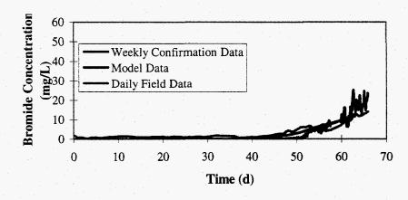
Figure 4-9: Comparison of Model Breakthrough to Field Breakthrough for EW-1
