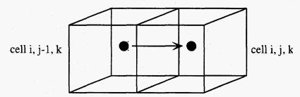
Figure 3-3: Flow through Cells in a Finite-Difference Grid (Adapted from McDonald and Harbaugh, 1988)
