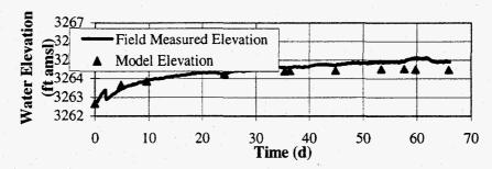
Figure 4-20: PV-2 Field and Model Groundwater Elevations
