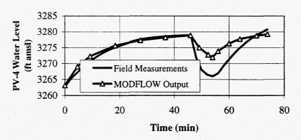
Figure 4-3: Water Elevations during Initial Injection Period at PV-4
