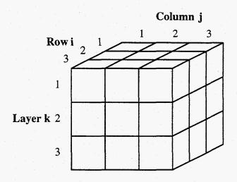
**Figure 3-1:** Row, Column, and Layer Configuration in a Finite-Difference Grid (Adapted from McDonald and Harbaugh, 1988)
