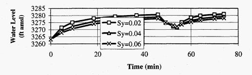
Figure 4-5: Sensitivity to Specific Yield in Initial Injection Model at PV-4
