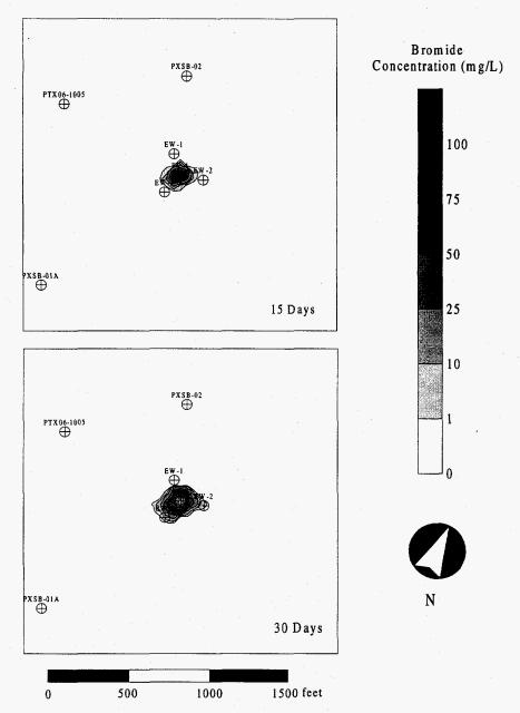
Figures 4-12 and 4-13: Bromide Contours for 15 and 30 Days of the Tracer Test
