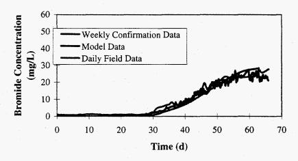
Figure 4-10: Comparison of Model Breakthrough to Field Breakthrough for EW-2
