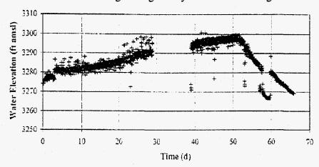
Figure 2-13: One Hour Moving Average of PV-4 Water Elevation
