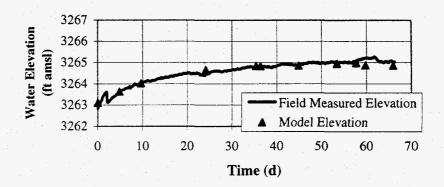
Figure 4-21: PV-3 Field and Model Groundwater Elevations
