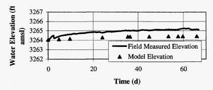
Figure 4-19: PV-1 Field and Model Groundwater Elevations
