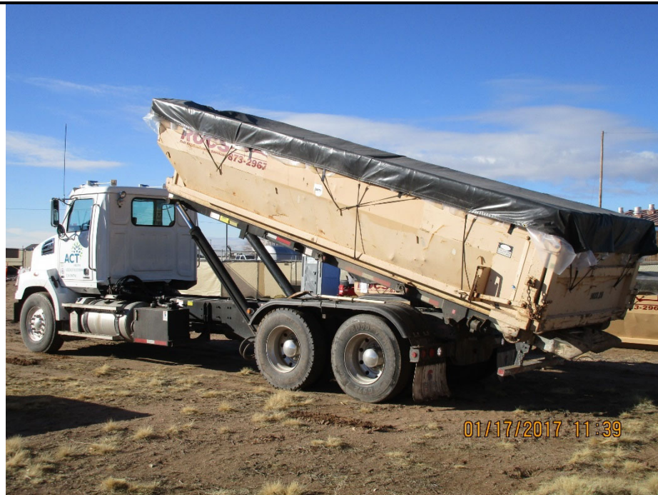
Description: ACT removing roll-off containing soil cuttings.
