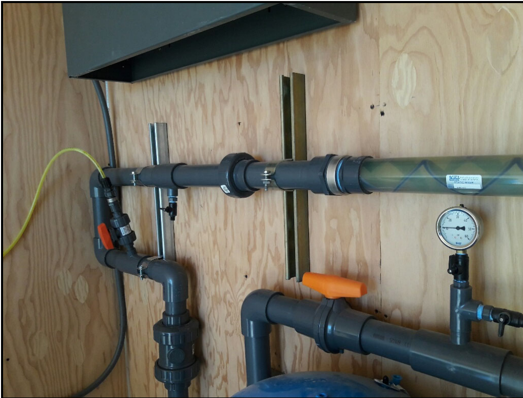
Description: Description: Fluorescein being introduced to the recirculated groundwater through the injection port, and flowing through the static mixer during Phase 1 tracer test.
