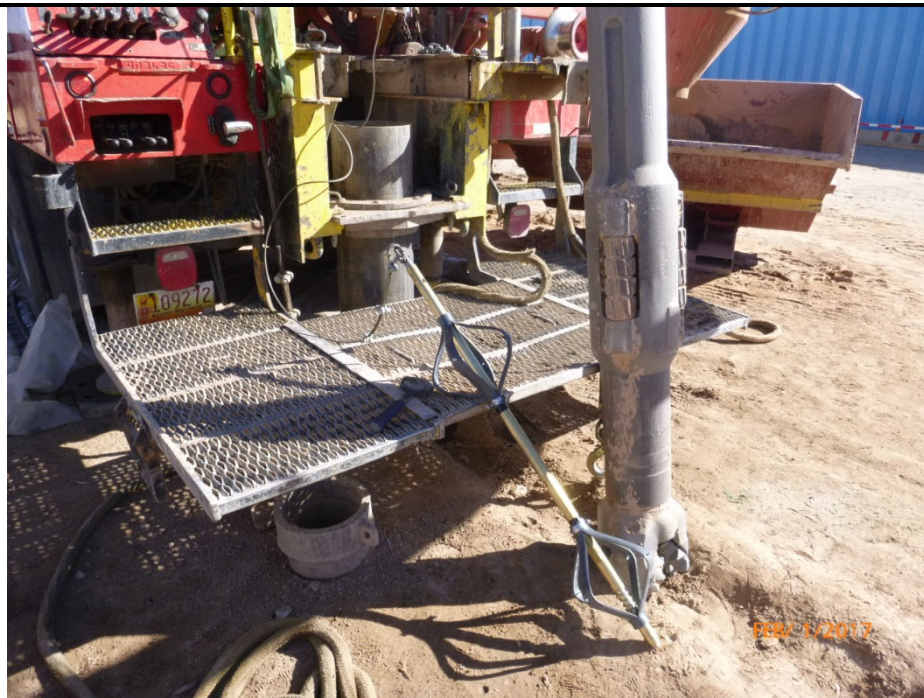
Description: EZ Trac ready for downhole deviation testing.
