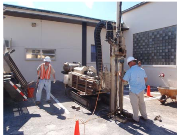
Figure 5.4. Schematic of Geoprobe MIP system, including use of the system during the ESTCP ER-201032 field demonstration (Source: Geoprobe SOP, 2012; http://geoprobe.com/literature/mip-logging-sop ).
