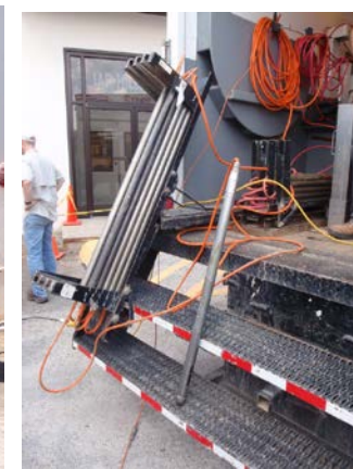
Figure 5.4. Schematic of Geoprobe MIP system, including use of the system during the ESTCP ER-201032 field demonstration (Source: Geoprobe SOP, 2012; http://geoprobe.com/literature/mip-logging-sop ).
