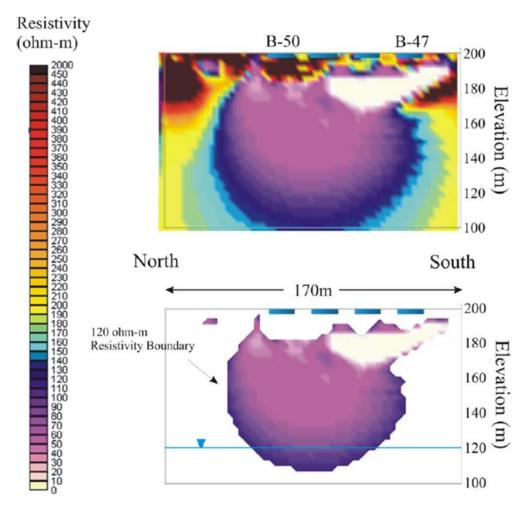
**Figure 28**. Electrical resistivity survey depicting a vertical slice of the subsurface where the low-resistivity region is expected to correspond with the vadose zone contaminant distribution (Serne et al. 2010).
