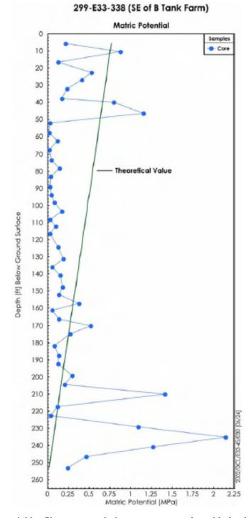
**Figure 19**. Matric potential by filter paper technique on core samples with depth along well 299-E33-338 (Serne et al. 2008; Lindenmeier et al. 2008).
