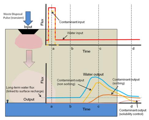
**Figure 31**. Generic description of the vadose zone as a transport path from the surface to groundwater for non-volatile contaminants.
