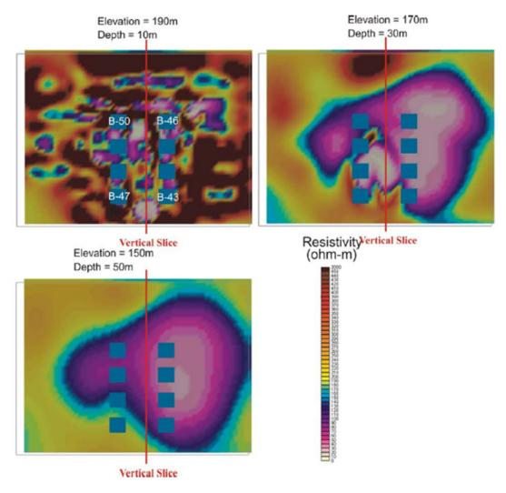
**Figure 27**. Electrical resistivity survey depicting lateral extent of low resistivity expected to correspond with the vadose zone contaminant distribution (Serne et al. 2010).
