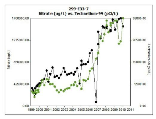
**Figure 30**. Groundwater concentrations over time of nitrate (black) and Tc-99 (green) at well 299-E33-7 in the BY area (Serne et al. 2010).
