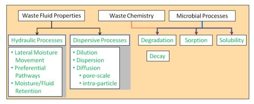
**Figure 8**. Attenuation mechanisms (green font) for inorganic contaminants in the vadose zone and factors that can impact attenuation (black font).
