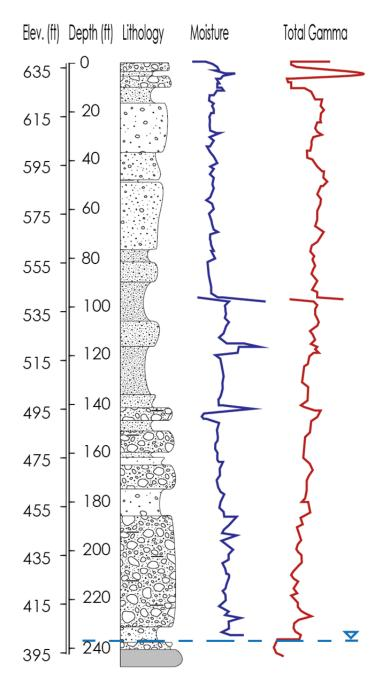
**Figure 26**. Lithology, total gamma, and water content versus depth for well 299-E33-342 in the BY area. Note that the low-permeability CCU is not present in this area.
