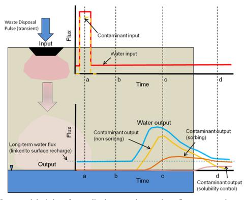
**Figure 5**. Conceptual depiction of generalized water and contaminant fluxes to groundwater resulting from a pulse input of water and contaminants to a vadose zone.
