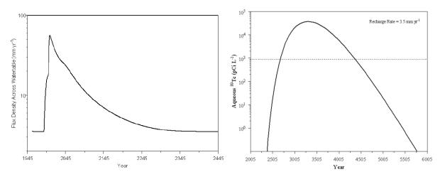
**Figure 24**. Simulated water flux across the water table (left) and predicted Tc-99 concentrations over time in the groundwater (right) beneath the trenches portion of the BC Cribs and Trenches site (Ward et al. 2004). The dashed line in the right plot is the Tc-99 drinking water standard. Note that the time scales are different on the two plots. Water flux has returned to recharge-driven conditions by about the year 2345 and the bulk of the Tc-99 enters the groundwater after that time.
