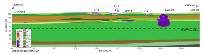
Figure 12. Differences in water saturation between 2007 and 1944 (initial) (Oostrom et al. 2008).
