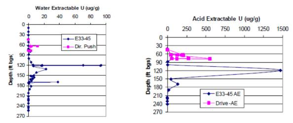
Figure 17. Water (A) and acid (B) extractable U concentrations with depth at BX-102 and at well 299-E33-45 (Serne et al. 2010).
