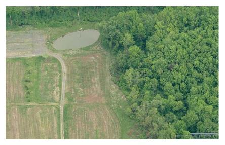
The U.S. Environmental Protection Agency excavated arsenic-contaminated soil from the parcels from summer of 2007 through the spring of 2009. Excavation of contaminated sediments in this spring-fed creek was completed in February 2009. The contaminated pond was filled to cap the contaminated sediments in place. This former pond and adjacent soil excavation area were then graded to create a wetland, which is fed by the spring that previously discharged to the pond.
