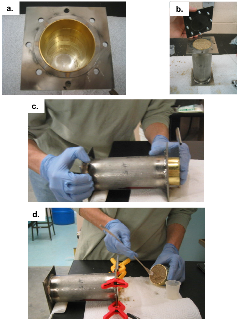
Figure 3.1. Refined core apparatus for examining MDE effects associated with different sampling methods and environmental conditions. Note: (a.) empty core with 7 brass rings inside; (b.) core packed with sand; (c.) extruding a brass ring from the core barrel; (d.) temporary cap on the core barrel while the brass ring is being sampled.
