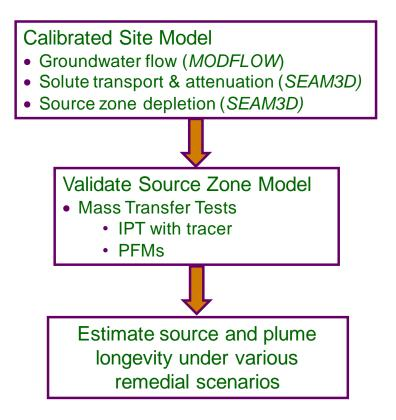
The field data are intended to provide input to a calibrated transport model. SEAM3D is an advective-dispersive numerical solute transport model that simulates the full range of natural attenuation processes in groundwater systems. SEAM3D also explicitly simulates the dissolution of a NAPL source zone based on fundamental mass transfer analyses and a calibrated SZD function for purposes of scaling the results from the TEE test scale to the entire NAPL zone at the site.
