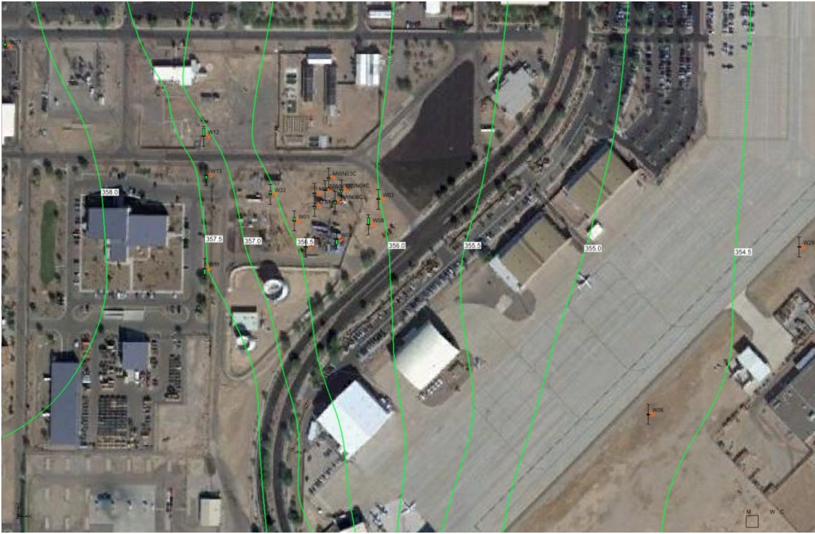
Figure F-3: Simulated Hydraulic Head Distribution in the LSZ and Calibration Targets for the ST012 Site Model.
