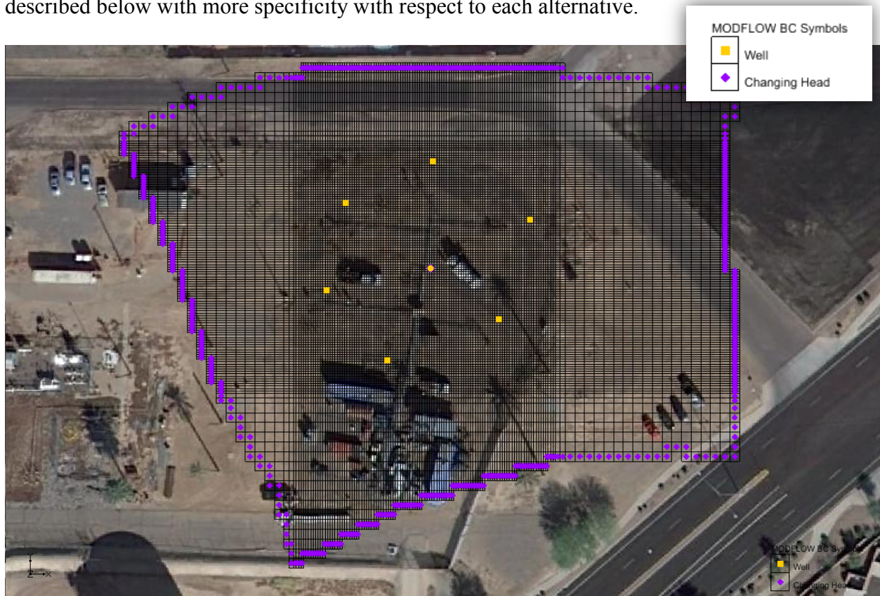
Figure F-6: Boundary conditions and sources and sinks in local-scale flow model.
