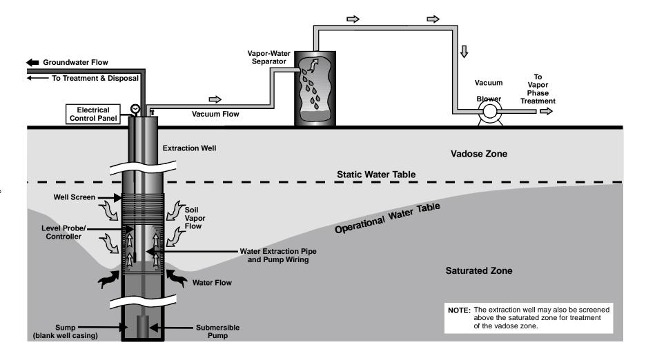
Figure 2. Schematic of a DPE System (Low Vacuum or High Vacuum)
