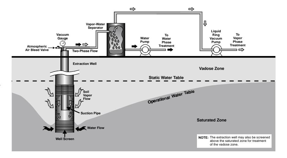
Figure 1. Schematic of a TPE System
